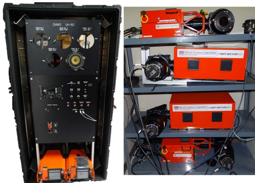
Figure 4. Bench top UMWS and Projectors
