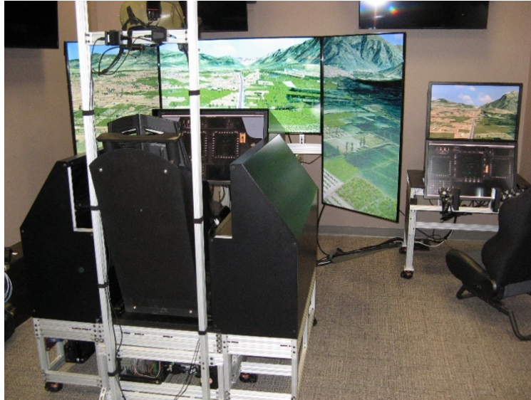
Figure 2. Virtual Cockpit Simulator
