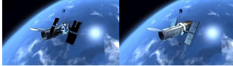
Figure 5. Vertex distortion at large distances with 32-bit floats (left) is resolved by using 64-bit floats (right).
