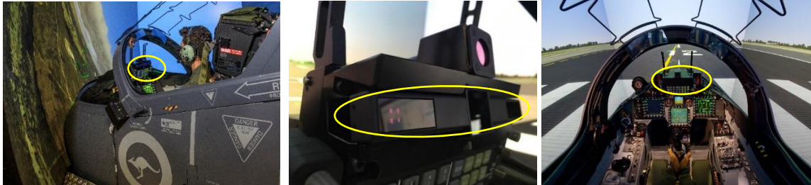
Figure 1. Hawk 127 Full Mission Simulator with Crew Training System installed (yellow highlight).
