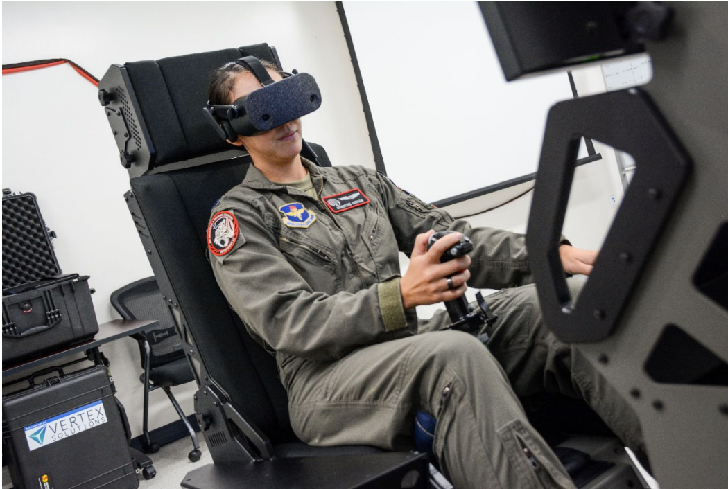
Figure 1. PTT station: VR headset, controls, displays. (Photo By: Aryn Lockhart, Air Force). The appearance of U.S. DoD visual information does not imply or constitute DoD endorsement.
