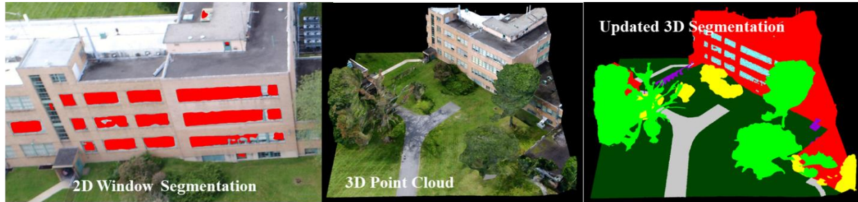
Figure 5. Image-based window segmentation results (left) are cast into the 3D point cloud model (center) to merge window segmentations with the other categories (right).
