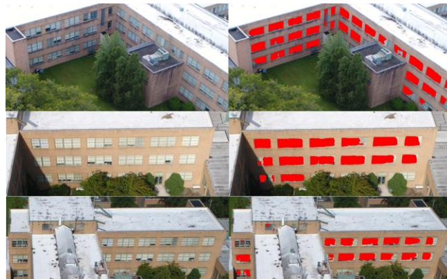
Figure 4. Image-based window segmentations using the presented pipeline. Window pixels are marked in red. Almost all instances of windows are detected accurately, even though the images are taken from an oblique, aerial view.
