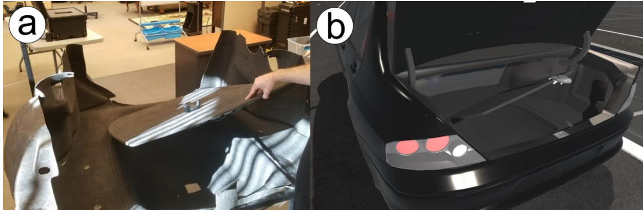
Figure 3. A Tier 1 physical trunk with a Tier 2 tracked wheel well cover (a) and the corresponding virtual view (b).
