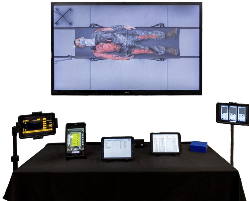
Figure 1. Shared components of an IMPACTT training system, including (clockwise from top) shared Virtual Patient, triple IV pump, IMPACTT Core (blue box), urine gauge, lab reports, ventilator, and patient monitor.
