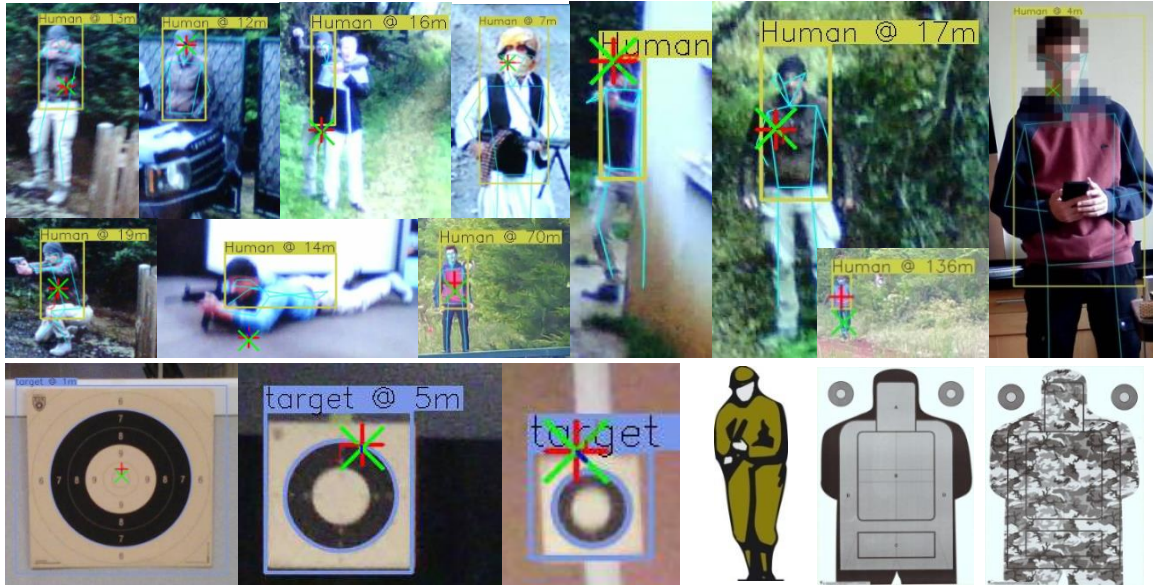
Figure 15: Detection example at different resolution (distance) and with various pose, occultation and camouflage.
