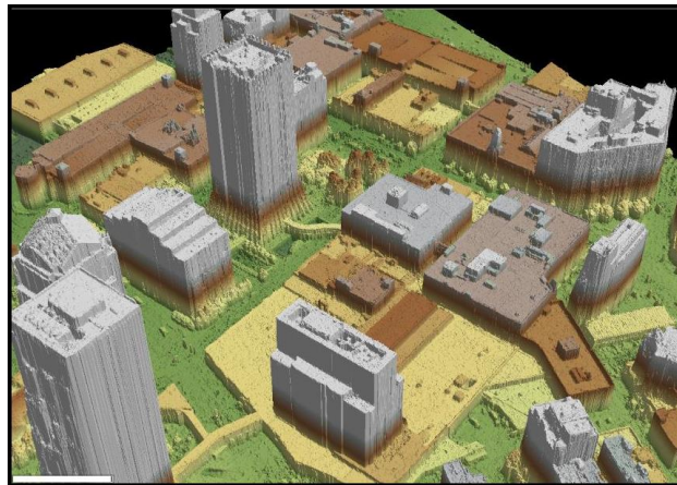
Figure 8. Extracted Digital Surface Model over Rochester, NY.
