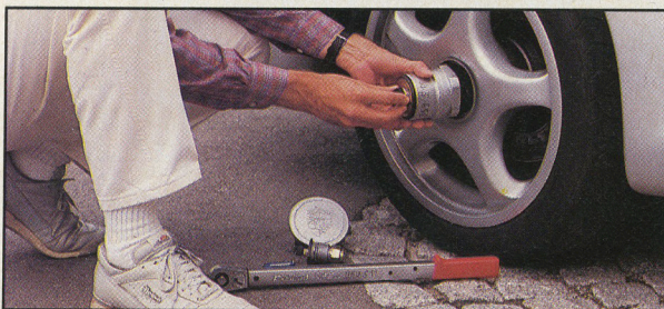
A small planetary gearbox and a preset torque wrench are used to apply the specified 625 pound-feet of torque to the wheels' central locking nuts.
