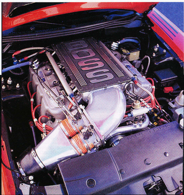
The Boss, with its big-box intake plenum and deeply contoured rocker covers, outpowered the Camaro.
