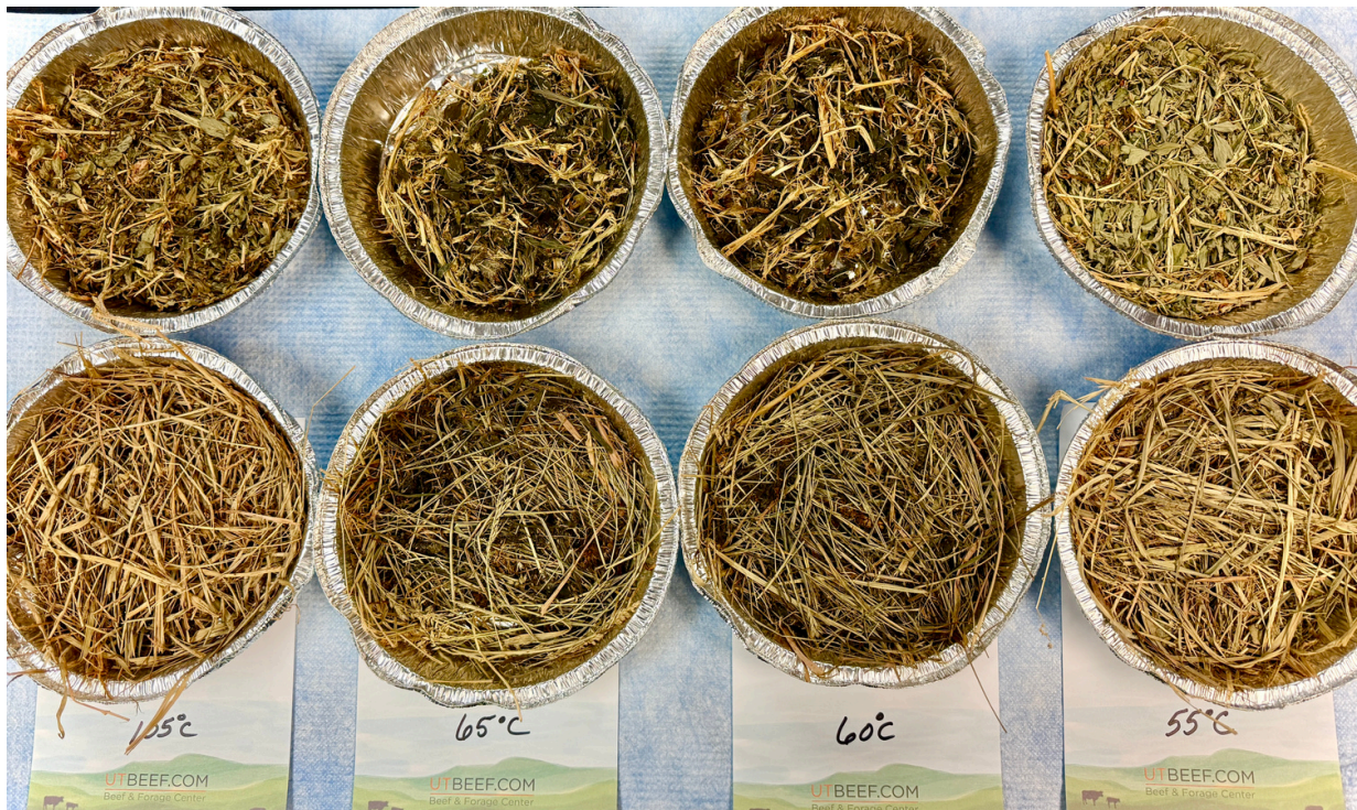
Fresh alfalfa and tall fescue samples dried at different forced air oven temperatures.
