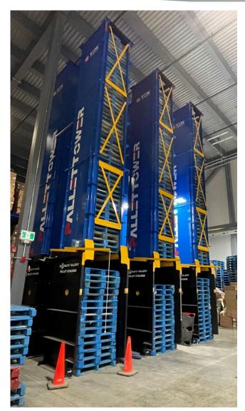
The Pallet Tower is a high density storage solution that stores up to 80 48"x40"CHEP pallets in a 5'x 5' footprint.
