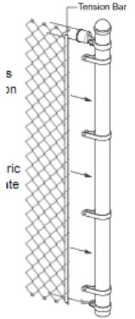
4. Gently crank the cable jack so that you begin to place tension on the wire. As you continue to crank the jack, stand the fabric up against the post. Pull the bottom of the fabric out away from the post approximately 6” to assure that it will not fall over. Note: Windy days and taller fabric may require temp ties or the fabric may need to be further pulled out away from the fence line.
