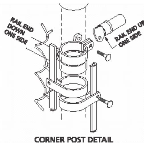
*How do I install the fittings?* Using the two charts to identify the fittings, you will install the fittings accordingly:
