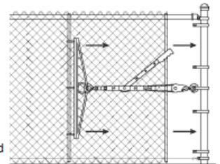
5. Once the fabric is all stood-up and the cable jack is taut, but not too tight. Pull the fabric from the far end of the fence line away from the cable jack by lifting it, shaking it and pulling it toward the cable jack. Repeat this every ten feet.
