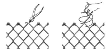
11. Complete this process of rolling-out fabric and weaving together until you have gotten to the next terminal post or 200’.
