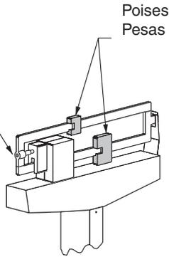
To balance scale, move both poises to zero (0) and turn balance screw to right or left until scale balances. For accurate weighing, place scale on level floor.
