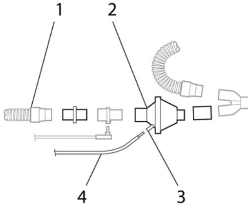
**Figure 3-9. Installing a pneumatic nebulizer**
