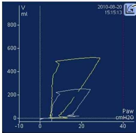
**Figure 7-8. Dynamic pressure/volume loop display**
