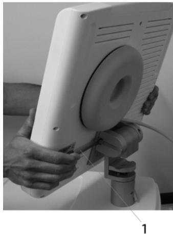
**Figure 2-4. Tilting the Ventilation Cockpit**
