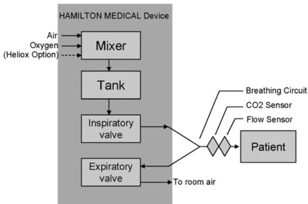
**Figure 1-4. Gas delivery in the device**
