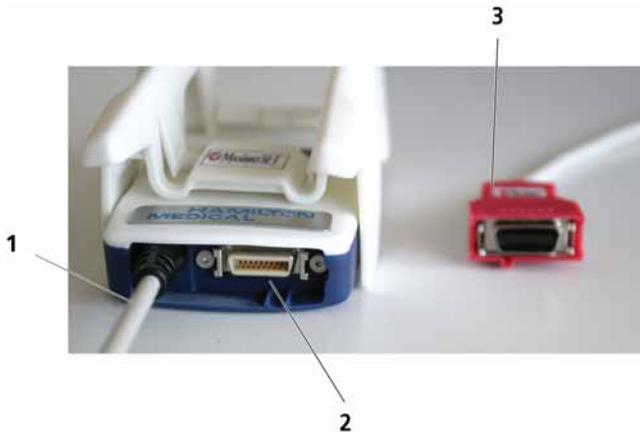
**Figure F-15. Masimo adapter and patient cables, connection ports on adapter**
