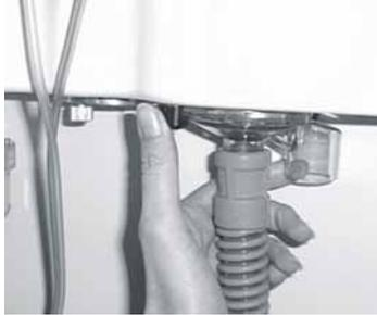
**Figure 2-16. Installing the expiratory valve cover**
