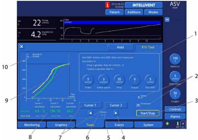
**Figure 9-3. P/V Tool window**
