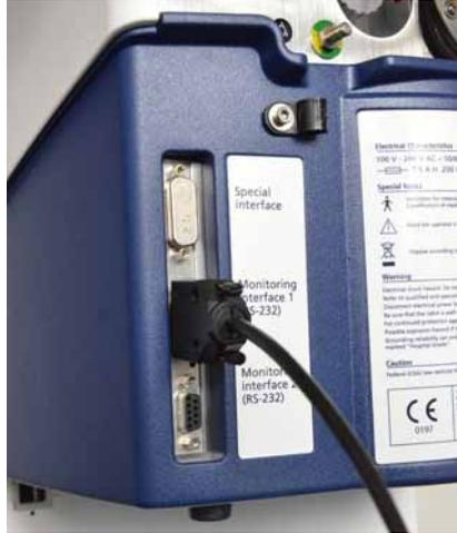
**Figure 2-9. HAMILTON-900 communications cable connected to RS-232 port on ventilator**
