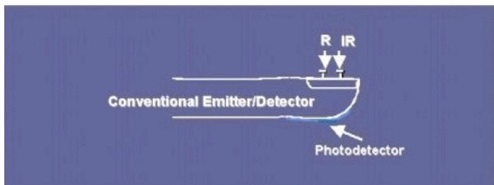
**Figure F-23. Scheme of a pulse oximeter**
