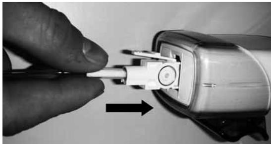
**Figure 3-7. Inserting the sample cell into the receptacle**
