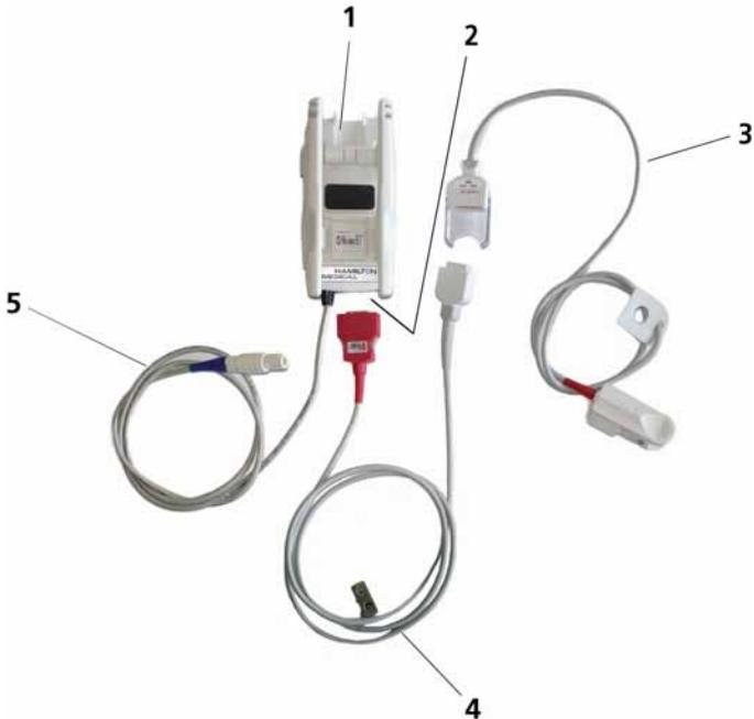
**Figure F-1. Masimo SpO<sub>2</sub> pulse oximeter components**
