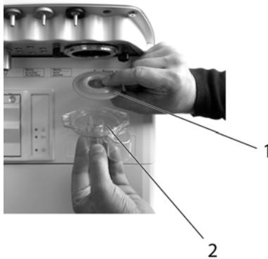
**Figure 2-15. Installing the expiratory valve membrane**
