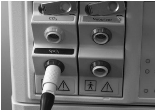
**Figure F-20. Connecting the patient cable to the ventilator**
