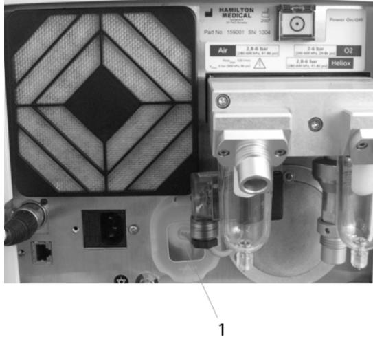
Figure 2-11. Check for the oxygen cell
