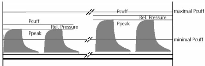
**Figure 3-27. Concept of automatically set  $P_{cuff}$  based on patient's airway pressure**
