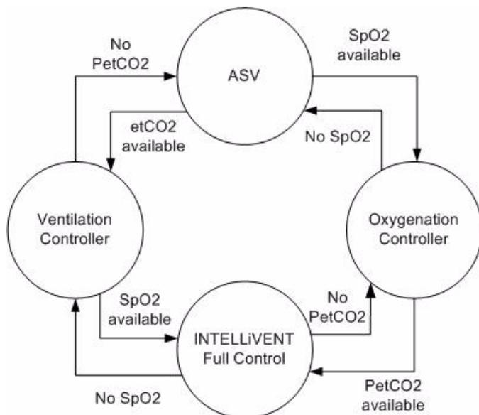
**Figure 1-2. Controller conceptual design**
