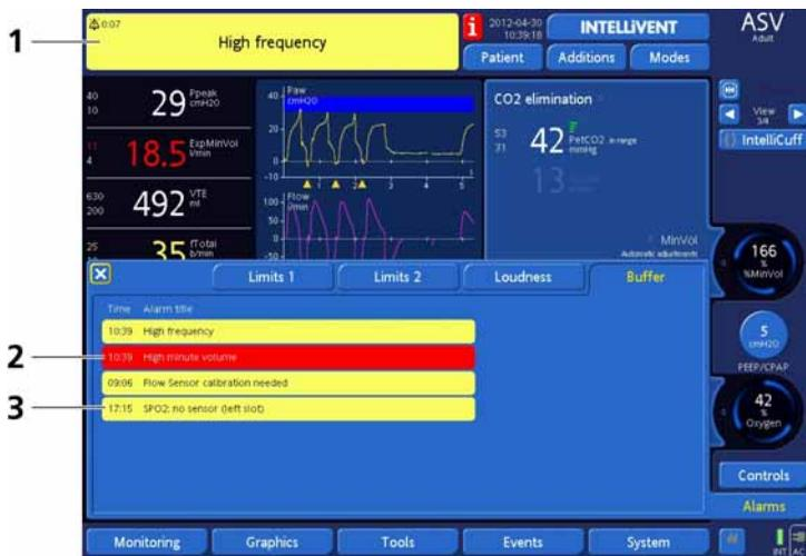
**Figure 10-2. Active alarm buffer**
