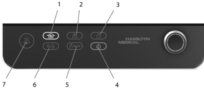
**Figure 12-1. Special function keys**
