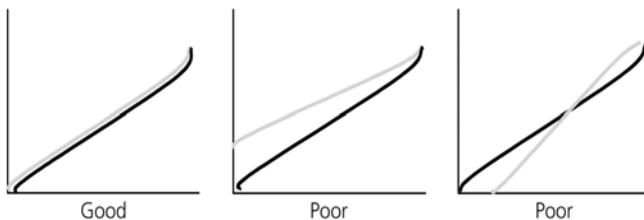
**Figure 9-12. Checking flow sensor performance**
