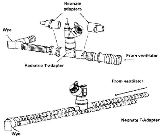
**Figure 3-17. Nebulizer for neonatal breathing circuit**
