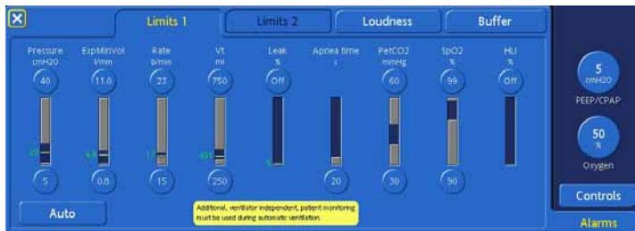
**Figure 5-10. Alarm Limits 1 window**
