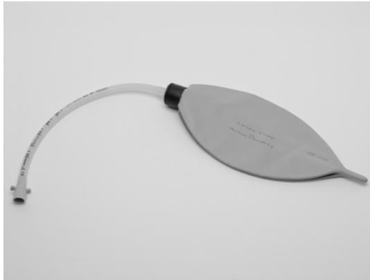
**Figure 9-10. Demonstration lung assembly**
