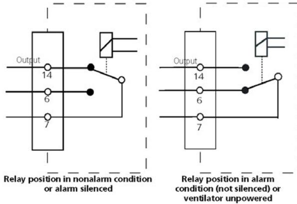
**Figure I-4. Remote alarm relay positions**
