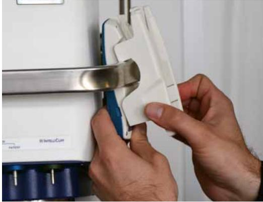
**Figure F-14. Fit adapter over rail**
