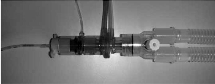
**Figure 3-8. Attaching the CO<sub>2</sub> sensor to the airway adapter**
