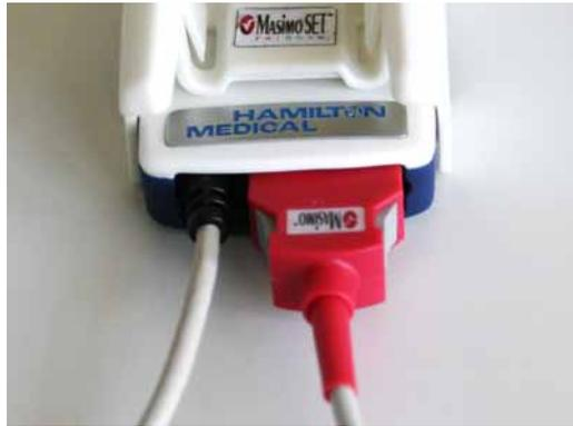
**Figure F-17. Connecting the patient cable to the SpO<sub>2</sub> adapter (Masimo)**
