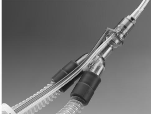
**Figure 2-17. Installing the flow sensor**
