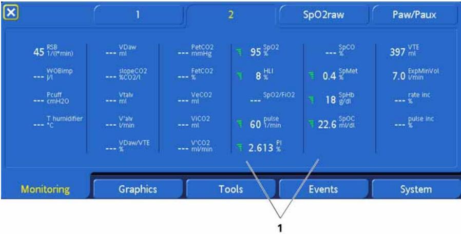
**Figure F-3. Monitoring window, Window 2 tab<sup>1</sup>**
