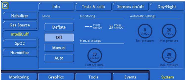
Figure 3-24. User Interface for automatic cuff pressure control (manual or no automatic adjustment activated)
