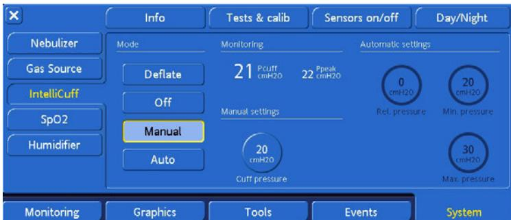
**Figure 3-25. User Interface for cuff controller, showing cuff pressure kept constant at manually set level.**
