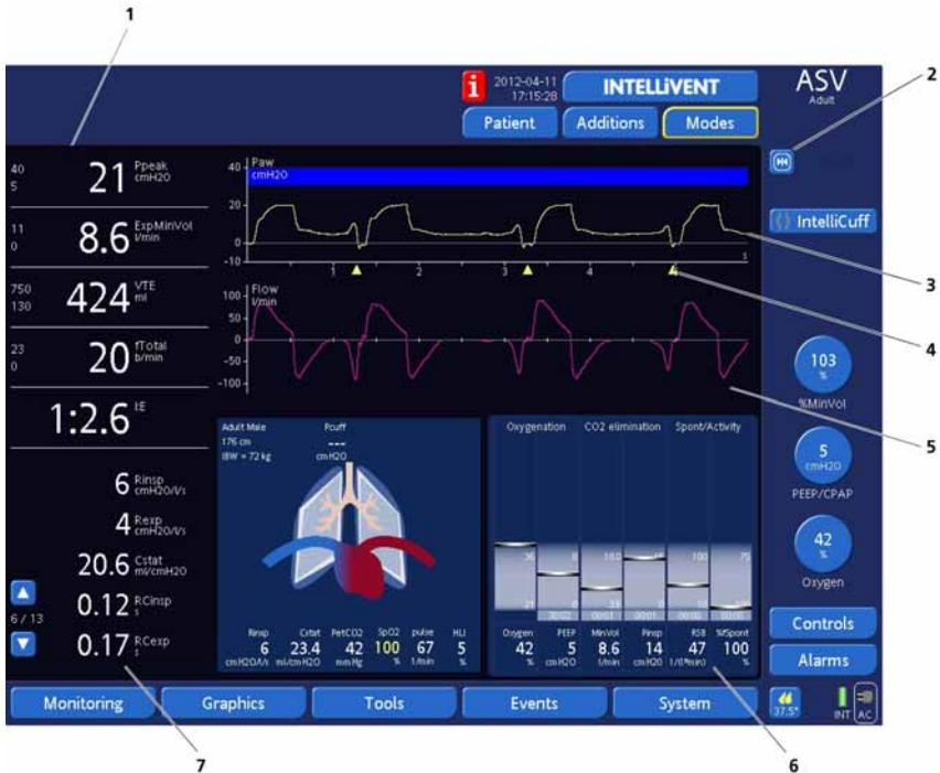
**Figure 7-1. Basic display with monitoring windows**
