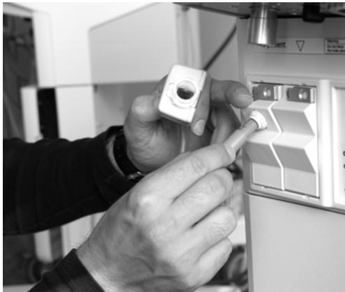
**Figure 3-2. Connecting the CO<sub>2</sub> sensor cable**
