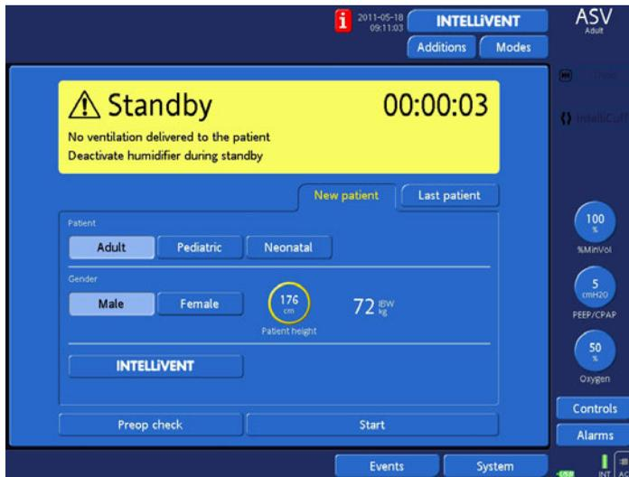
**Figure 12-3. Standby activated window**
