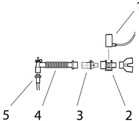
**Figure 3-4. Connecting the CO<sub>2</sub> sensor/airway adapter to the patient circuit**
