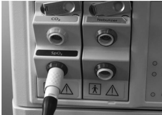
**Figure F-16. Connecting the ventilator SpO<sub>2</sub> cable to the ventilator (Masimo)**
