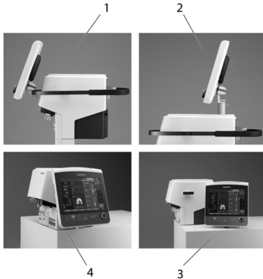
**Figure 2-1. Ventilation Cockpit mounting positions**
