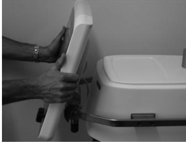
**Figure 2-3. Mounting the Ventilation Cockpit**
