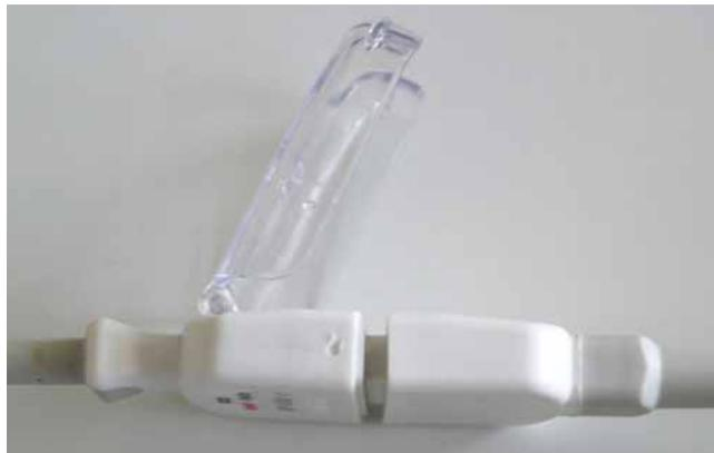
**Figure F-18. Connecting the patient cable to the sensor (Masimo)**
