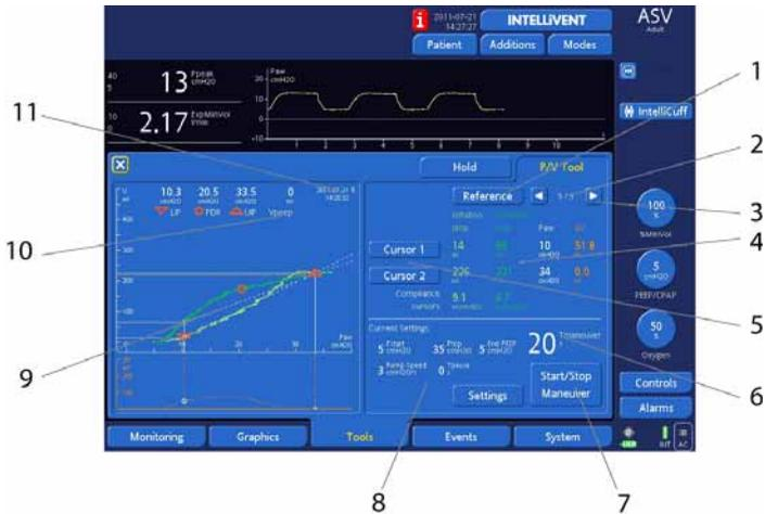
**Figure 9-4. P/V Tool Pro window**
