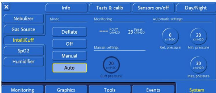
Figure 3-26. User Interface for cuff controller, cuff pressure automatically adapted to actual airway pressure
