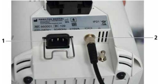
**Figure 2-8. Power, communication connections (bottom)**
