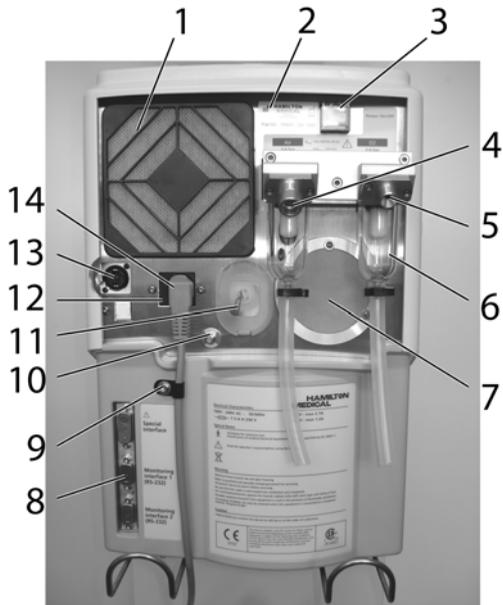
**Figure 1-11. Rear of ventilation unit**
