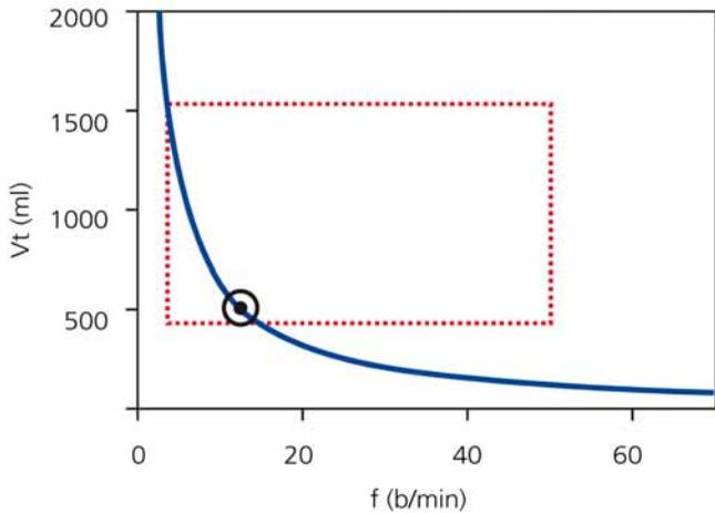
**Figure C-9. Anatomy of the ASV target graphics window.** The rectangle shows the safety limits; the circle shows the target breath pattern.
