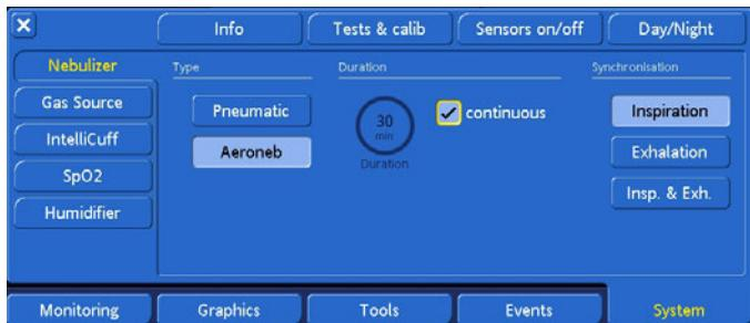
**Figure 3-20. Continuous nebulization**
