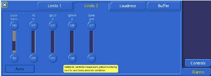
Figure F-5. SpO<sub>2</sub> Alarm Limits 2 window
