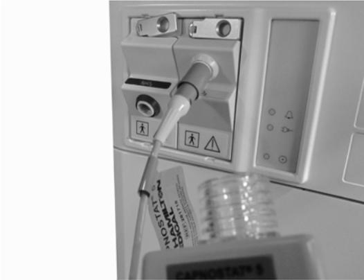
**Figure 4-4. CO<sub>2</sub> sensor/adapter calibration setup**
