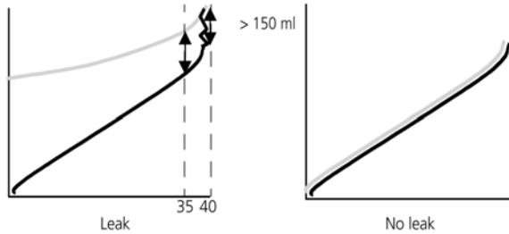
**Figure 9-11. Checking for a gas leak between the Flow Sensor and the demonstration lung**
