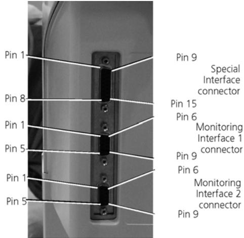
**Figure I-5. Interface connectors**
