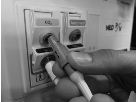
**Figure 3-6. Connecting the CO<sub>2</sub> sensor cable**
