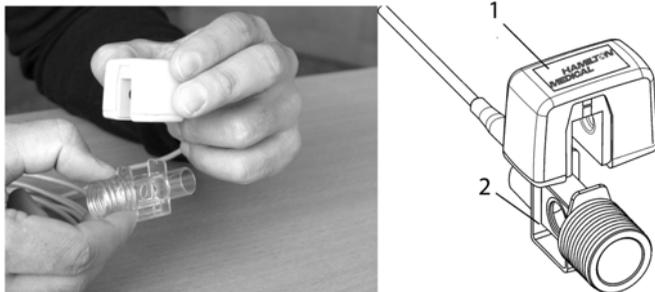
**Figure 3-3. Attaching the CO<sub>2</sub> sensor to the airway adapter**
