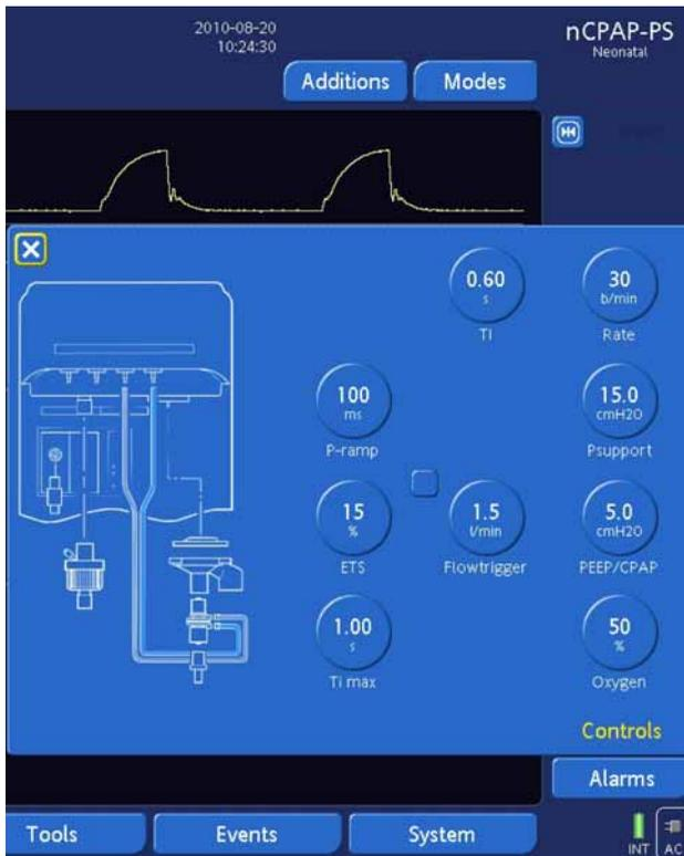
Figure B-17. nCPAP-PS basic controls
