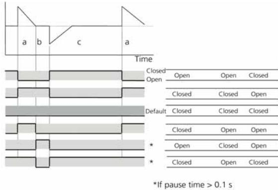
**Figure J-13. I:E outlet timing**
