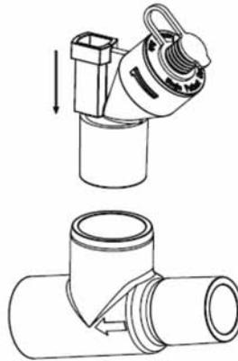
**Figure 3-12. Connecting nebulizer to T-adapter**
