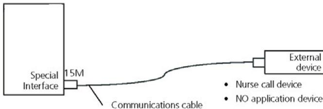
**Figure I-3. HAMILTON-G5 connected to an external device through the Special Interface connector**
