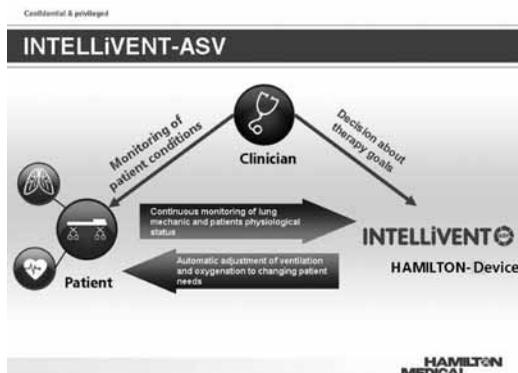
**Figure 1-1. Closed-loop ventilation**
