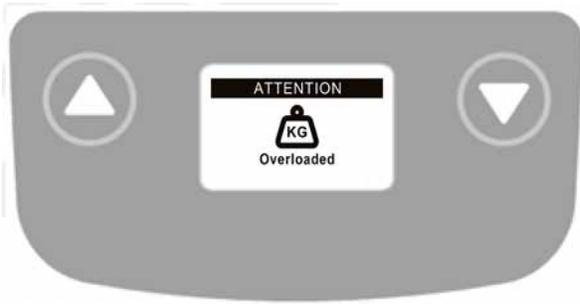
During lifting if the lift is overloaded, the LCD Display Panel will show the sign on the left and lifting will be deactivated immediately.
