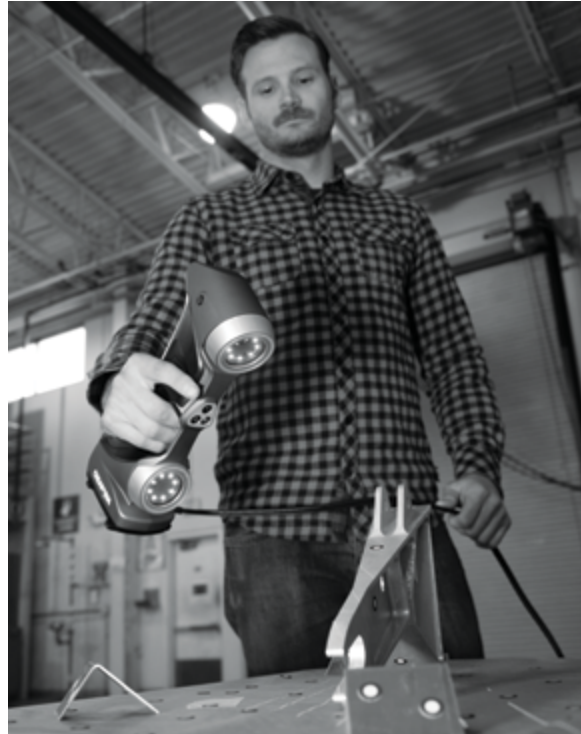
Joshua Orr, 60th Aircraft Maintenance Squadron, uses a CreaForm HandyScan 700 to capture digital information to render a three-dimensional image of an aircraft part into specialized computer software, Nov. 16, 2018, at Travis Air Force Base, California. The scanner will be utilized in conjunction with two additive manufacturing units, one polymer and one metal, to print aircraft parts on site. (U.S. Air Force Photo by Heide Couch).
