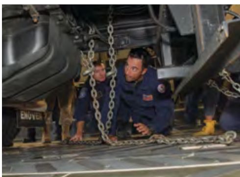
Liam McGregor, left, transportation manager and Matt Gonzales, California Urban Search and Rescue Task Force 7 transportation specialist, use a chain to secure an equipment transport trailer to the deck of a C-17 Globemaster III during a joint inspection and logistics drill conducted with 60th Aerial Port Squadron personnel June 13, 2019 at Travis Air Force Base, California. (USAF photo by Heide Couch).
