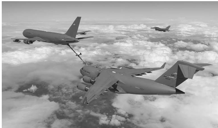
The KC-46 Pegasus refuels a C-17 Globemaster III July 12, 2016. The successful mission tested the hydraulic pressure relief valves installed to correct higher-than-expected axial loads in the boom. (Courtesy Photo)
