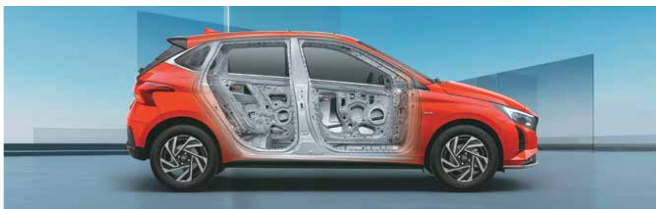
Strong body structure (with AHSS and HSS)
