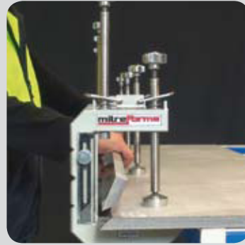
Place the fascia in position and ensure it is correctly aligned
