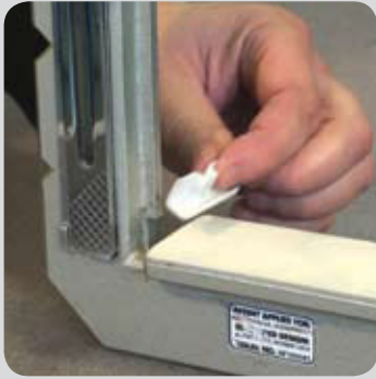
Insert glue-catcher in the rebate of the mitreForma™
