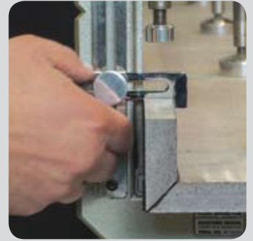
Use the retaining arms to ensure fascia is held firmly against the back guide
