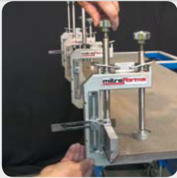
Use the fascia clamping rods to press the fascia into place. DO NOT over-tighten!
