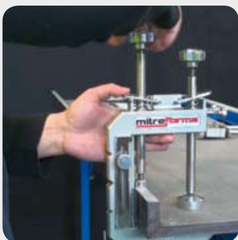
Unscrew the fascia clamping rods, then press the quick-release tab and retract the rod
