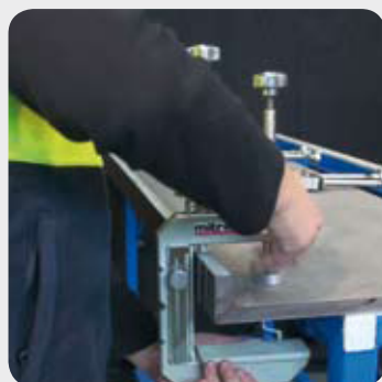
Unscrew the main clamping rod, then press the quick-release tab to lower and remove the mitreForma™
