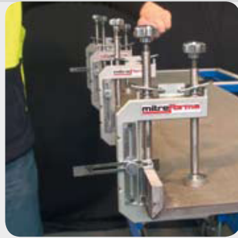
Check that all main clamping rods are firm and all the seams are correctly aligned
