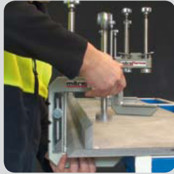
Place mitreForma™ in position using the quick-release rod, then screw until finger-tight
