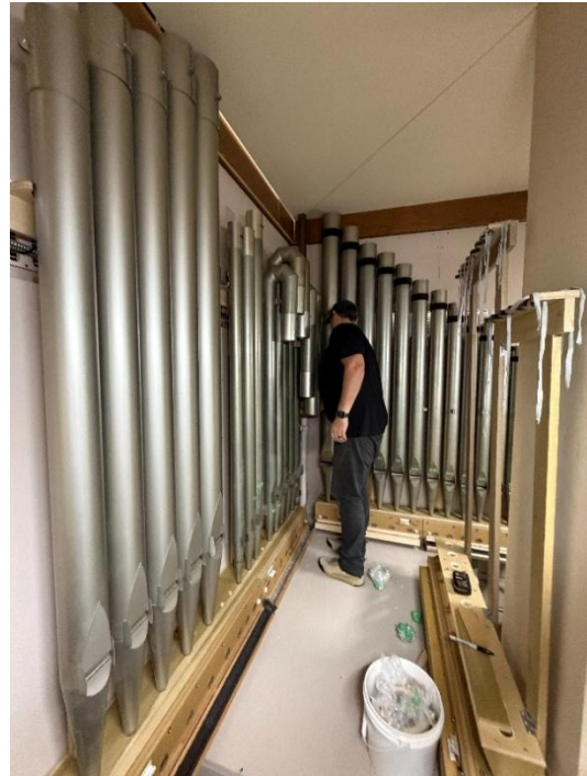
Above: Zac wires windchests under the Great Division which is in the middle of the pipe loft in front of the upper and lower Choir enclosures. There is not much room to work!
