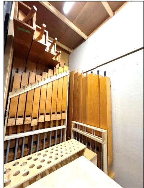
Bourdon pipes in place at the north end of the Swell enclosure. For efficient use of the space, the mitered pipes fit over the shorter pipes and the pipes in front have “long toes” with PVC wind extenders so they don’t block the sound of the pipes behind them.
