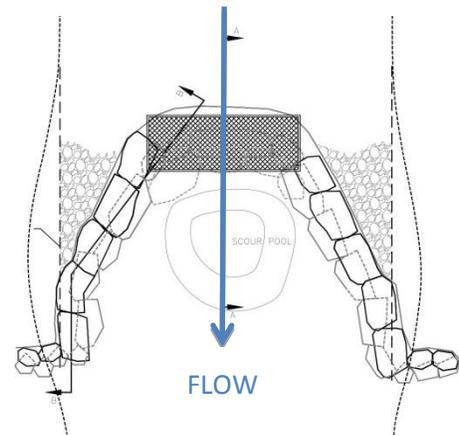
**Figure 1. Rock Drop Structure.**
