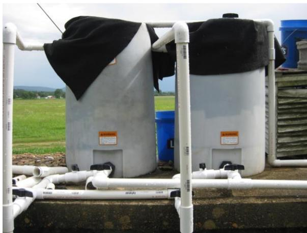
**Figure 5. Treatment #2 Filter Design.**
