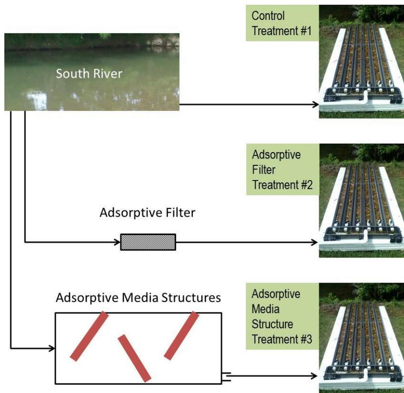
**Figure 4. Experimental Mesocosm Design.**
