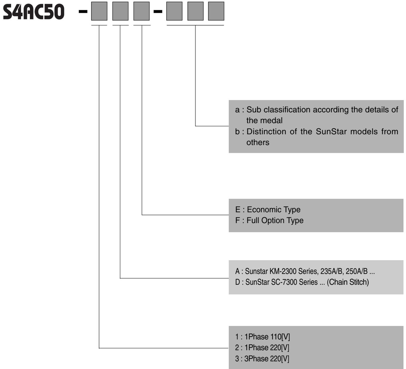
ORDER Ex. S4AC50-2AF refers to SERIES4, 1Phase 220V, FULL FUNCTION CONTROL BOX for normal drop feed.
