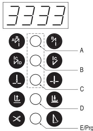
Turn the power on by simultaneously pressing the buttons , A and B, C.
