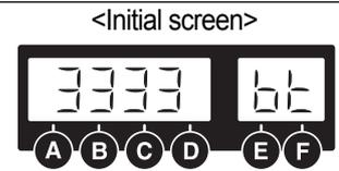
④ If you have checked the sewing condition, first correct the stitch number that differs by one or more stitches to the programmed stitch number.
