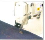
Top thread is taken up as soon as thread trimming is done.
