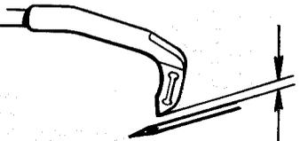
For denim sewing, push the needle 0.02 mm.
