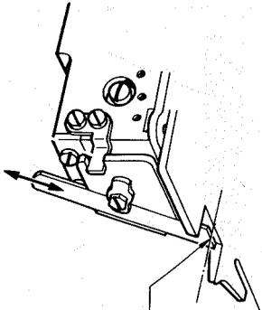
Align the tip of the lower knife with the needle plate surface.
