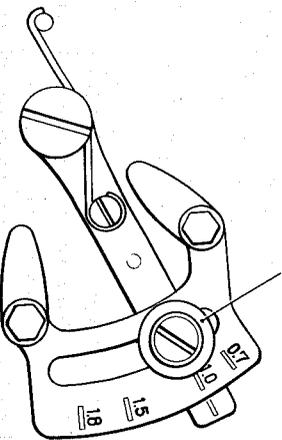
Loosen the set screw and adjust.
