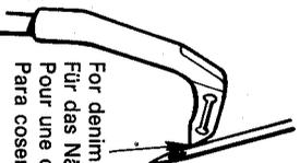
3. Adjust after aligning the lower looper hook point with the needle center in the needle lift stroke.
