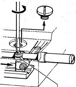
Loosen the needle bar clamp. Vertically shift, and turn the needle bar to adjust.
