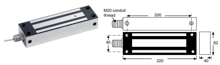
The EXM12-24 magnetic lock is totally sealed in an epoxy sealed stainless steel case with 20mm conduit for water-resistant and vandal-resistant purpose. It can be applied with access control.
