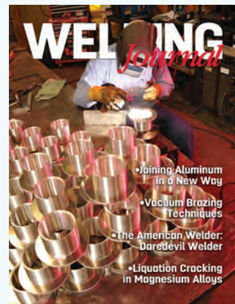
On the cover: A Dynamic Fabrication journeyman gas tungsten arc welds aluminum aircraft spacers. (Courtesy of Dynamic Fabrication, Inc., Santa Ana, Calif.)
