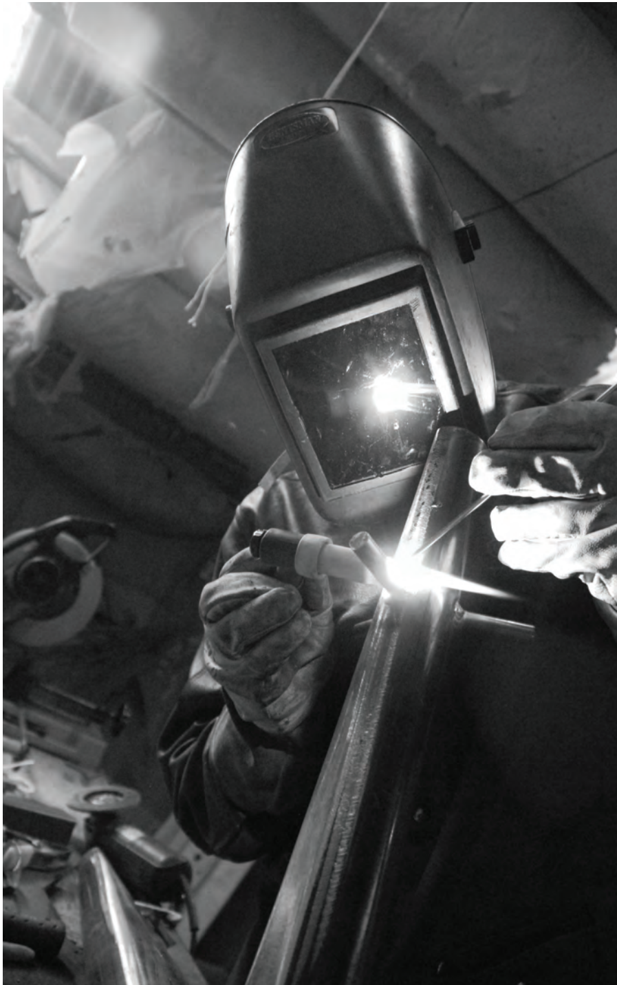
Fig. 3 — Gas tungsten arc welding a component for a sculpture. Photo courtesy of James Autery.
