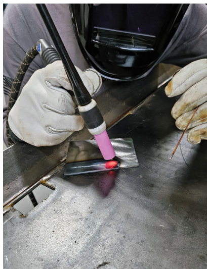
Maintain torch position during postflow to protect the hot tungsten and weld area.
