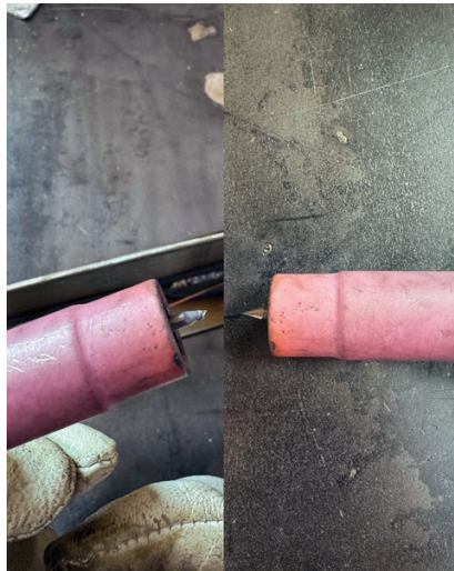
A contaminated (left) vs. clean (right) tungsten electrode.
