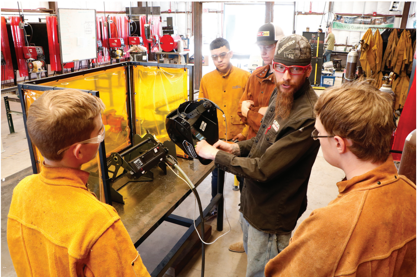
Fig. 2 — Marana High School Welding Instructor Kenton Webb explains to his students how to use a live welding training tool to fine-tune their welding techniques in the booth. The tool provides video game-like guides inside the welding helmet to guide students as they practice.
