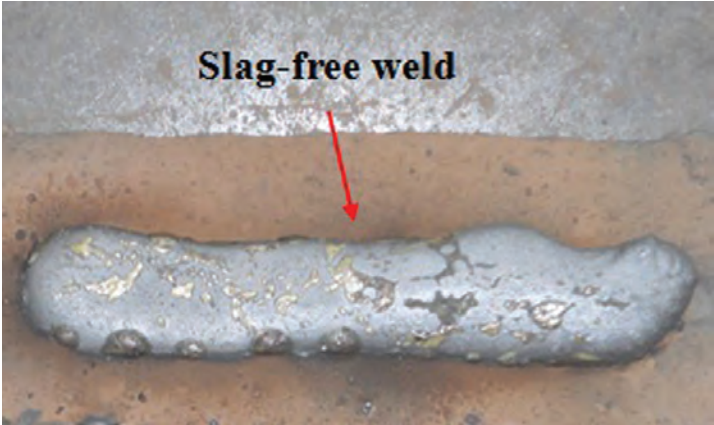
Fig. 2 — Typical weld appearance of the hardfacing alloy deposited by slag-free, self-shielded flux-cored wire.
