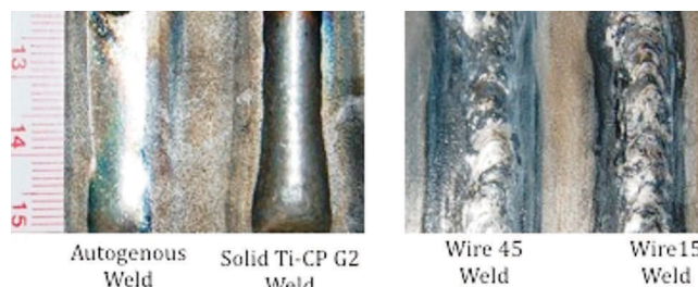
Fig. 2 — As-welded GTA (autogenous and solid wire) and A-TIG welds (Wires 15 and 45).
