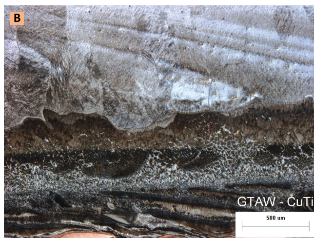
Fig. 6 — General microstructure observed in the Fe-Cu-Ti weld overlay deposited with a combination of CSC-GMAW and GTAW-P processes. A — Macro, B — Microstructure at the Cu-Ti interface, C — Microstructure of the 2 nd Ti layer.
