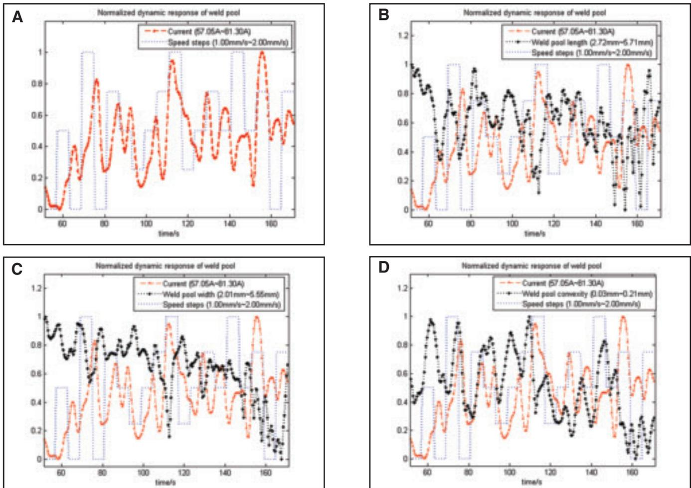
Fig. 1 — Identification experiment. A — Current and speed; B — length, current, and speed; C — width, current, and speed; D — convexity, current, and speed. All variables are plotted using the normalized scale. The range for each variable is given in each plot and corresponds to [0, 1] in the normalized scale.
