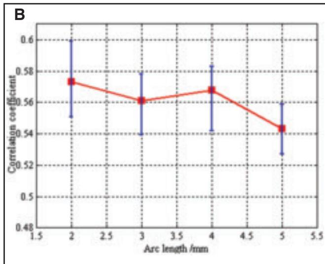
Fig. 10 — Standard deviations and correlation coefficients of the model using data from the verification experiments at different arc lengths. A — Standard deviation of the model; B — correlation coefficients of the model.
