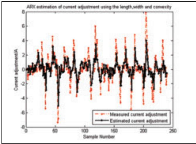
Fig. 6 — Estimation of the welder's response using the ARX model that uses all three characteristic parameters.
