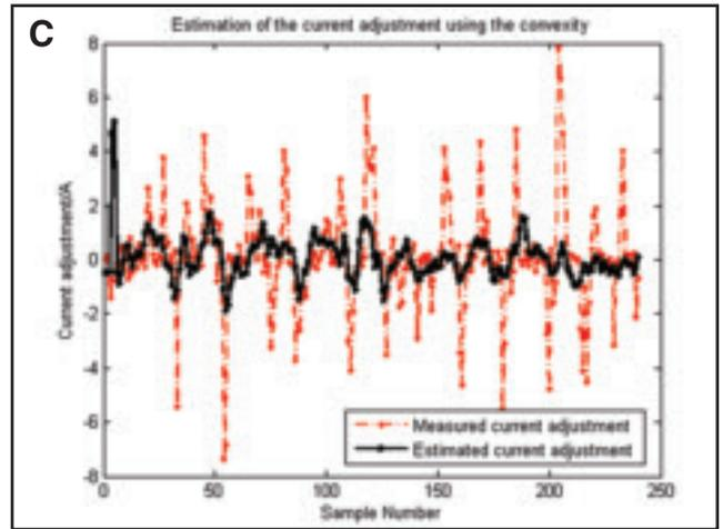
Fig. 3 — Estimation of the welder's response using the models with the single input. A — Estimation using the length; B — estimation using the width; C — estimation using the convexity.
