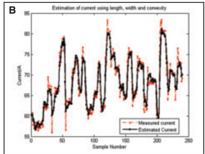
Fig. 5 — Estimation of the welder’s response using the models with three inputs. A — Estimation of current adjustment; B — estimation of current.
