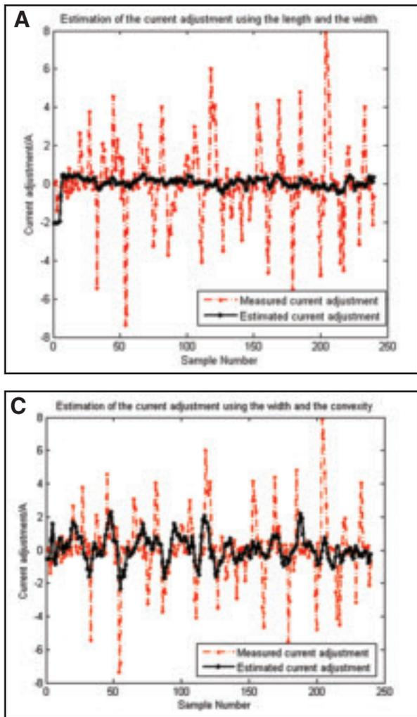
Fig. 4 — Estimation of the welder's response using the models with two inputs. A — Estimation using the length and width; B — estimation using the length and convexity; C — estimation using the width and convexity.
