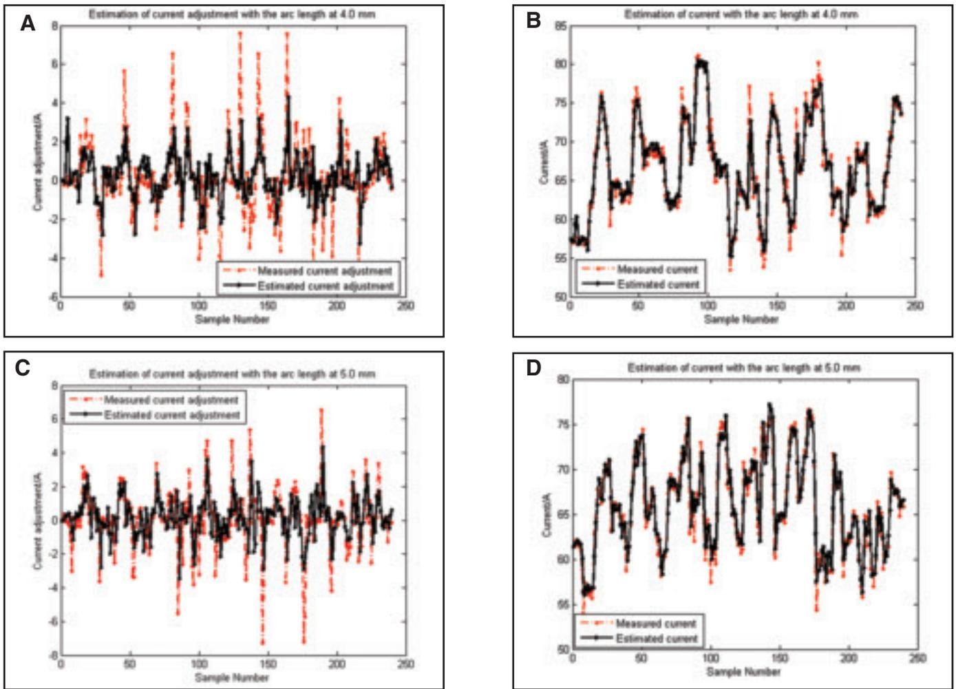
Fig. 9 — The prediction of the human welder’s response using model  $H_{lwh}(z)$ . A — Estimation of current adjustment with arc length 4.0 mm; B — estimation of current with arc length 4.0 mm; C — estimation of current adjustment with arc length 5.0 mm; D — estimation of current with arc length 5.0 mm.
