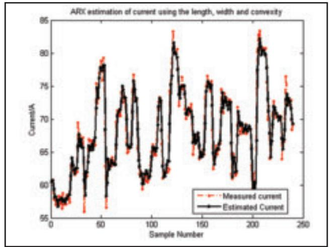
Fig. 7 — Comparison of the ARX model estimated welding current with the measured current. The ARX model makes use of the width, length, and convexity calculated from the 3D weld pool surface as the weld pool characteristic parameters, and the previous adjustments on the welding current to predict the welder's adjustment on the welding current.
