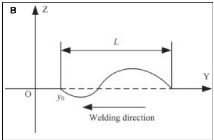
Fig. 4 — Weld pool modeling and parameters. A — 2D boundary; B — longitudinal intercepted area.
