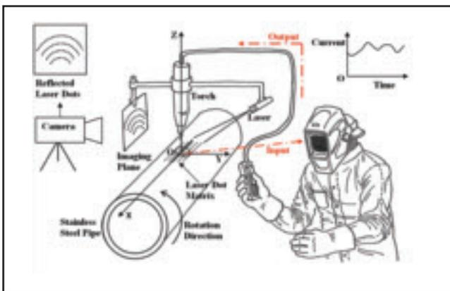
Fig. 5 — Demonstration of a manual control system featuring the GTAW process. The use of the remote control for welding current shown in the figure is for demonstration purposes only. The actual current remote control is a thumb turn knob on the torch. It adjusts the current setting for the power supply.
