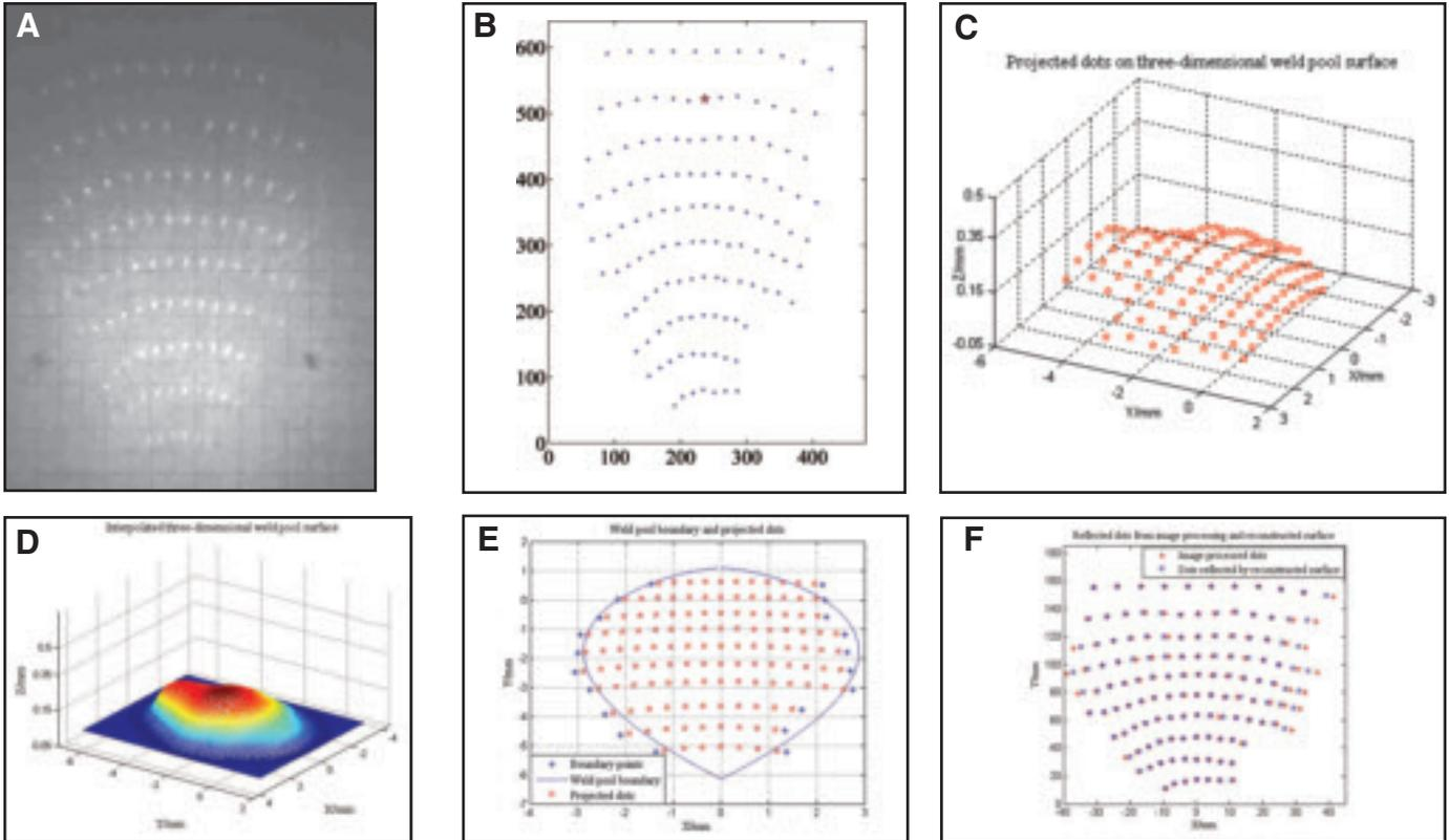
Fig. 3 — Results of image processing and 3D reconstruction. A — Captured image using the sensing system; B — resultant dots in the captured image using image processing; C — projected dots on the 3D weld pool surface; D — interpolated 3D weld pool surface; E — weld pool boundary and the projected dots; F — measured and calculated reflection pattern.
