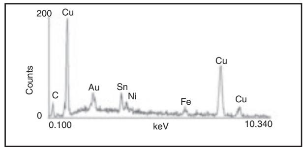
Fig. 10 — EDS analysis of a small area component of the brazing alloy-to-Kovar interface (Region G).
