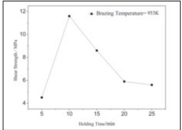
Fig. 4 — Relationship between the brazing time and shear strength.
