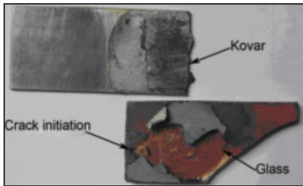
Fig. 5 — Macromorphology of shear crack on a brazed joint.
