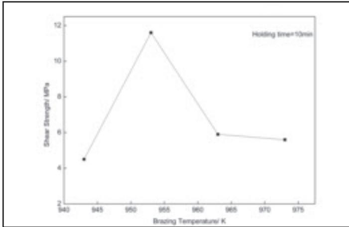
Fig. 3 — Relationship between the brazing temperature and shear strength.
