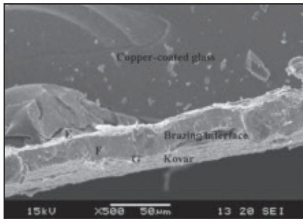
Fig. 7 — Microstructure of the joining interfaces for glass/brazing alloy/Kovar alloy.
