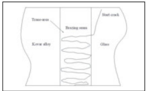
Fig. 6 — Map of rupture crack path of a brazed joint.
