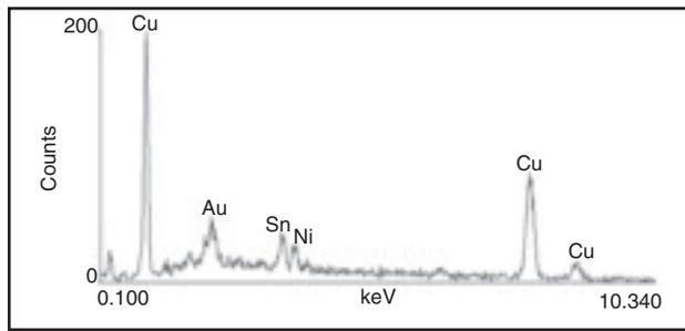
Fig. 9 — EDS analysis of a small area component of the brazing alloy (Region F).
