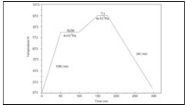
Fig. 2 — Technical requirement graph of the vacuum brazing experiment.
