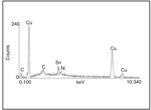
Fig. 8 — EDS analysis of a small area component of the glass-to-brazing alloy interface (Region E).
