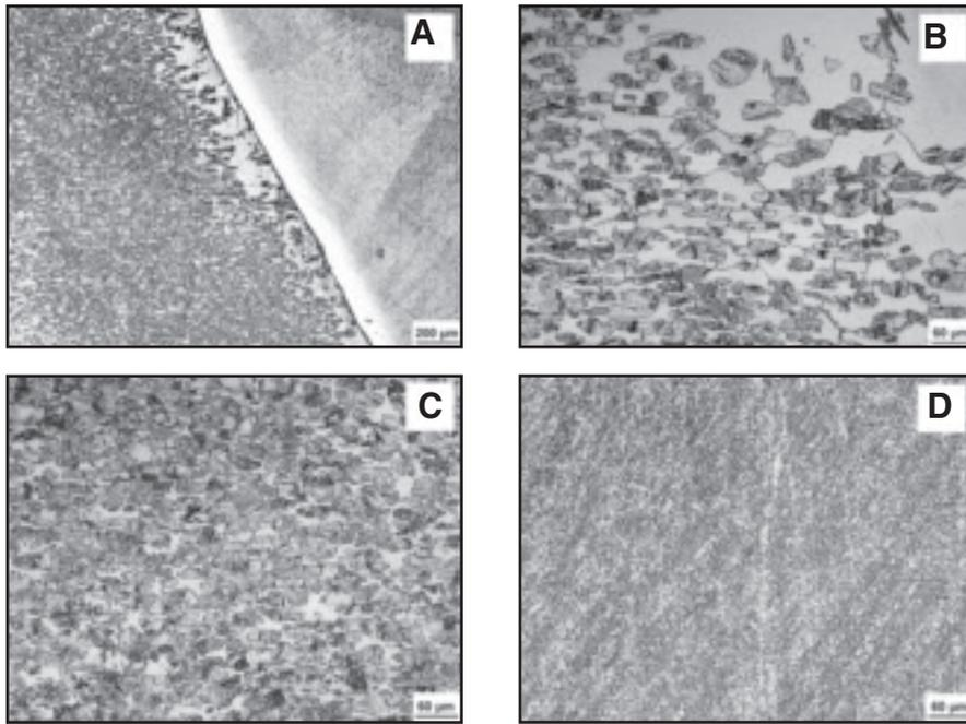
Fig. 4 — Photomicrographs of GMA weld with 316 filler metal (B6). A — WM+HAZ, 50 $\times$ ; B — HAZ, 200 $\times$ ; C — LTHAZ, 200 $\times$ ; D — WM, 200 $\times$ .
