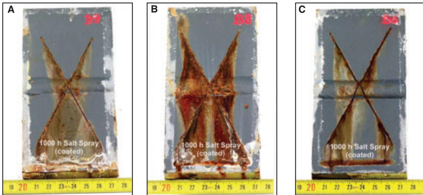
Fig. 9 — Coated salt spray corrosion test samples after 1000 h. A — B9; B — B8; C — B6.
