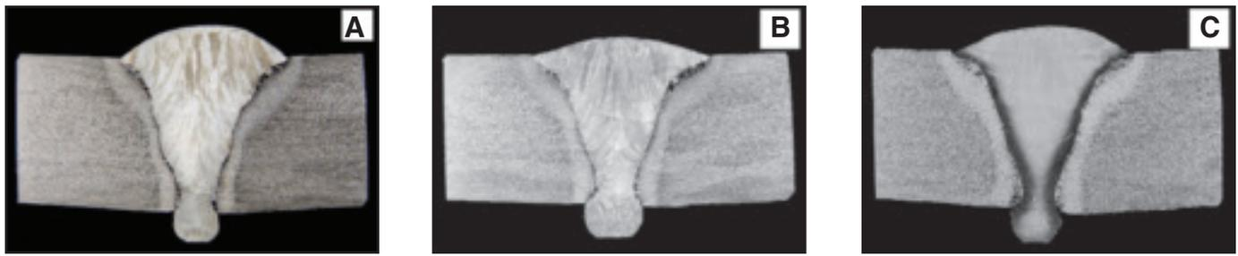
Fig. 1 — Photo macrographs of welded joints. A — B9; B — B8; C — B6.
