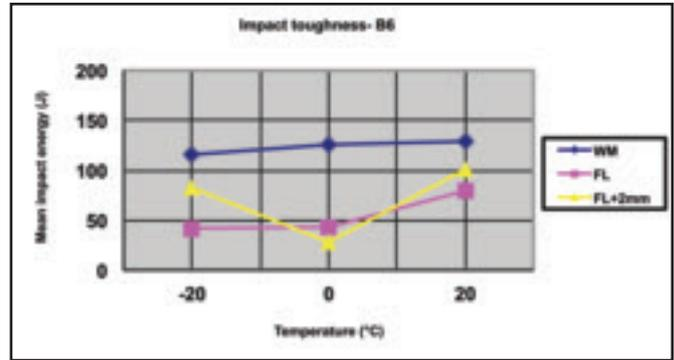
Fig. 5 — Notch impact toughness of the GMA welded joints (B9, B8, and B6).
