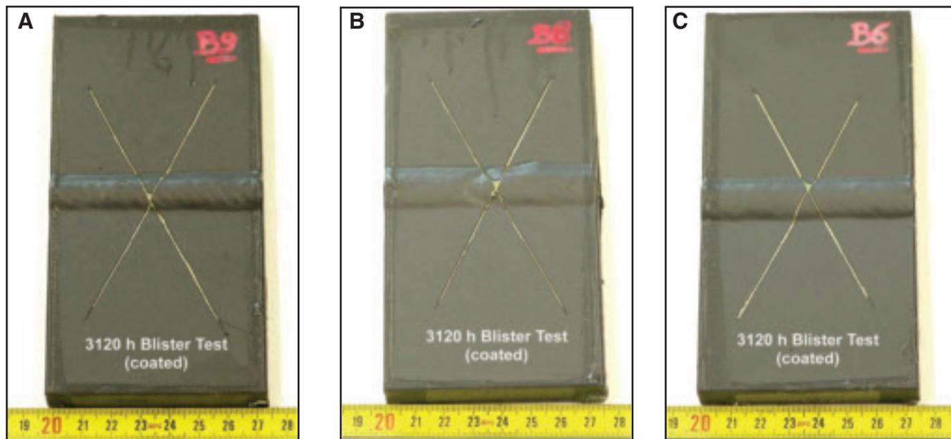
Fig. 11 — Coated blister corrosion test samples after 3120 h. A — B9; B — B8; C — B6.
