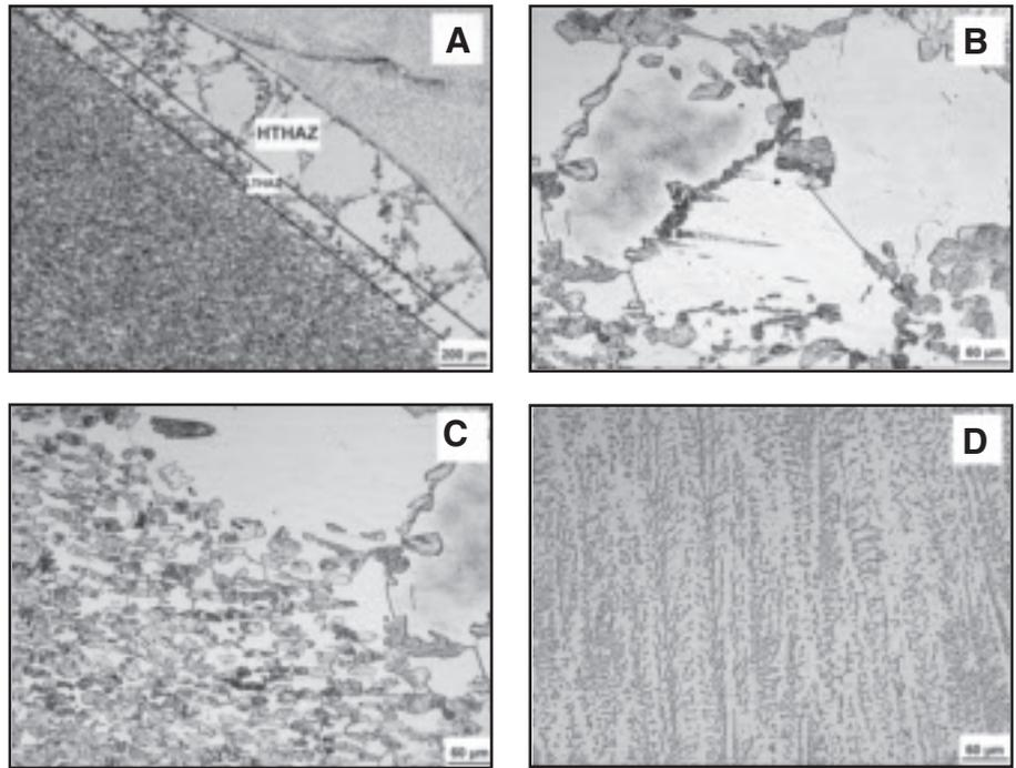
Fig. 3—Photomicrographs of GMA weld with 308 filler metal (B8). A—WM+HAZ, 50x; B—HTHAZ, 200x; C—HAZ, 200x; D—WM, 200x.
