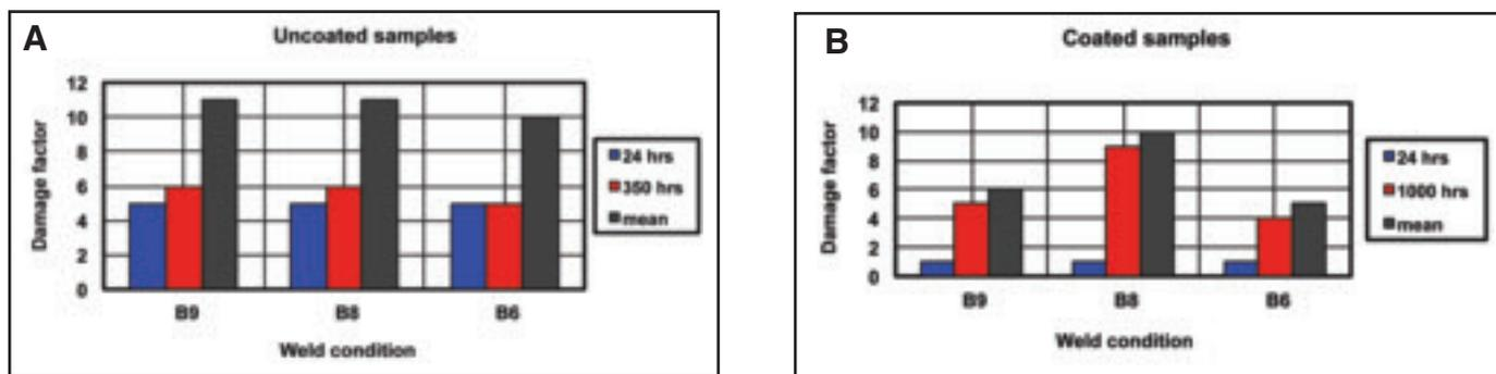
Fig. 10 — Damage factor during salt spray corrosion test. A — After 24 and 350 h for uncoated samples; B — after 24 and 1000 h for coated samples.
