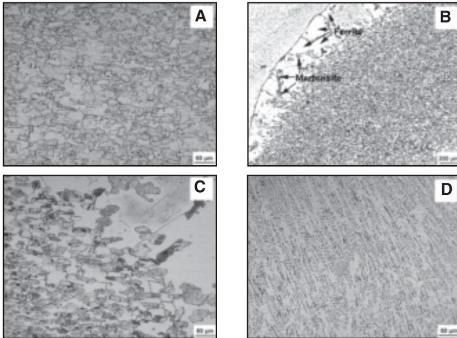
Fig. 2 — Photomicrographs of GMA weld with 309 filler metal (B9). A — BM, 200x; B — WM+HAZ, 50x; C — HAZ, 200x; D — WM, 200x.
