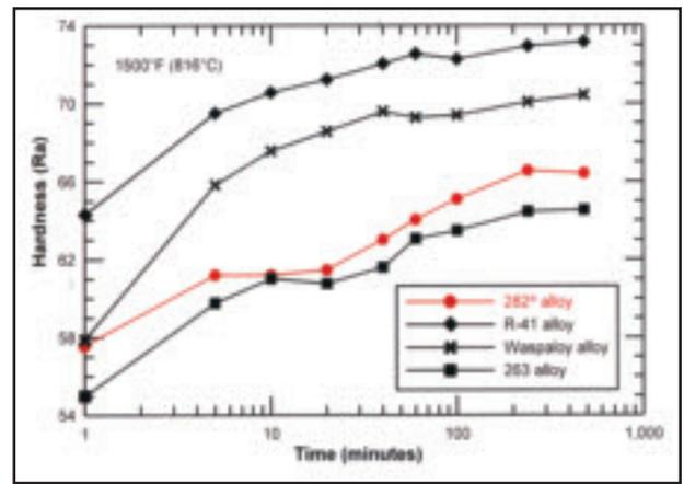
Fig. 7 — Comparative age-hardening kinetics of several wrought gamma-prime-strengthened alloys (Ref 8).
