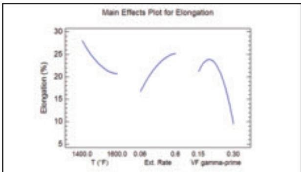
Fig. 3 — Main effects plot for CHRT elongation as function of temperature, extension rate, and equilibrium gamma-prime volume fraction.
