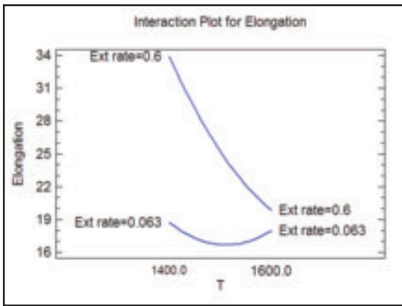
Fig. 6 — Extension rate/test temperature interaction plot.
