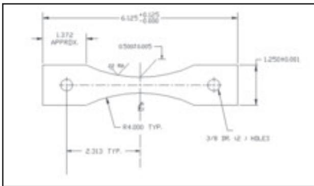
Fig. 1 — Specimen geometry used in CHRT response surface experiment.
