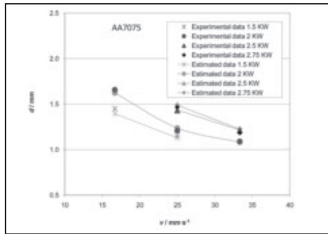
Fig. 8 — Measured and estimated penetration values (*d*) of 6082 butt joints, in function of the processing rate (*v*) and the laser power (*P*).
