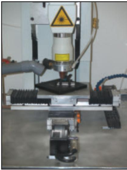
Fig. 1 — Laser equipment and mobile X-Y table.
