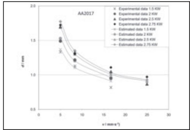
Fig. 4 — Measured and estimated penetration values ( $d$ ) of 1050 butt joints, in function of the processing rate ( $v$ ) and the laser power ( $P$ ).
