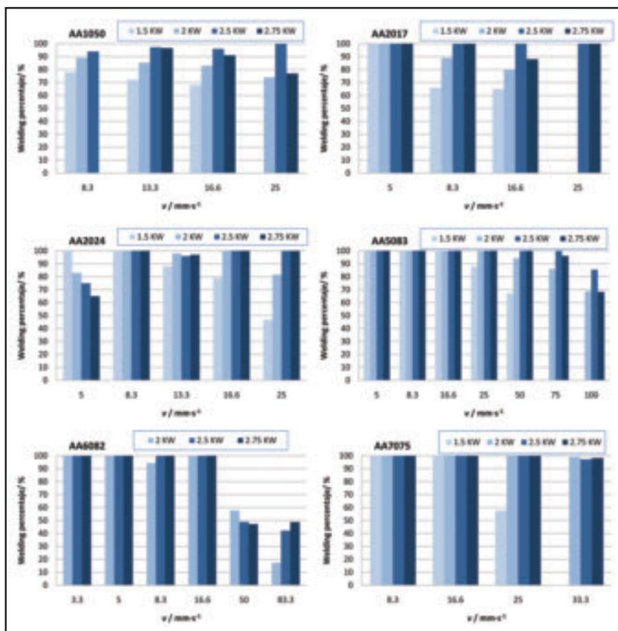
Fig. 3 — Welding percentage of aluminum alloys as function of the welding speed ( $v$ ) and the laser power ( $P$ ).
