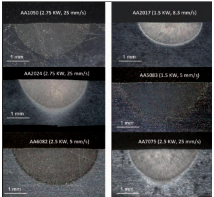
Fig. 2 — Examples of metallographic images (30×) of butt-joint weld beads in aluminum alloys, obtained with the indicated laser power and welding rate conditions.
