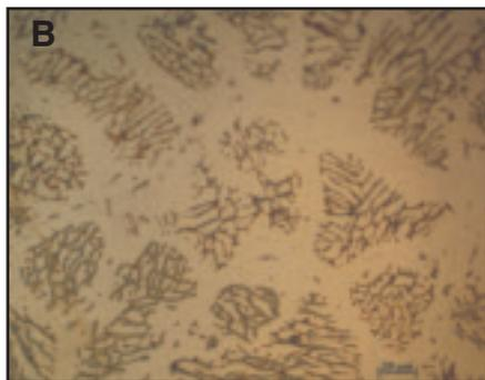
Fig. 9 — Ferrofluid EMG 911 on FA. A — Sample A32, skeletal ferrite morphology; B — Sample A57R, lathy ferrite morphology.
