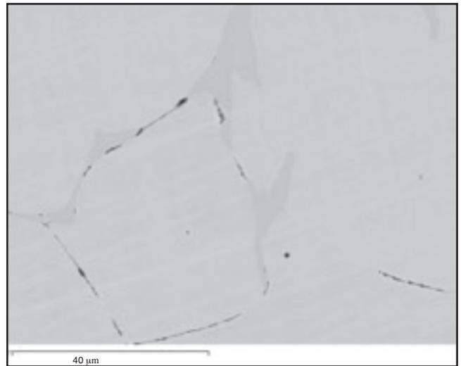
Fig. 2 — Faint contrast between austenite and ferrite. Fry's reagent.
