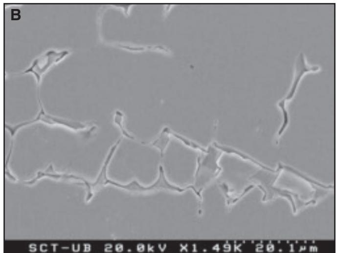
Fig. 3 — Oxalic acid etching on sample A31. A — SEM equipment; B — FEG-SEM equipment.
