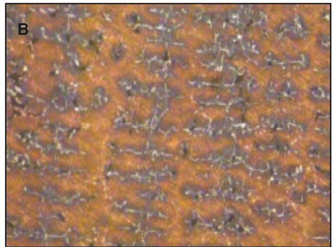
Fig. 4 — Lichtenegger-Blöch etching on sample A31. A — 30 s, hot (500x); B — 45 s at boiling (200x).
