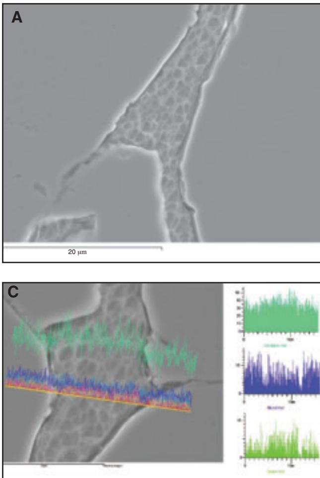
Fig. 5 — Beraha's etching on sample A31. A — Micrograph; B — spot microanalysis inside the  $\delta$ -ferrite dendrite; C — linear microanalysis.
