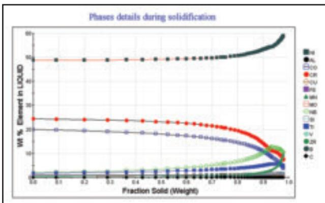
Fig. 8 — Predicted segregation of elements in the liquid as a function of the fraction solid.
