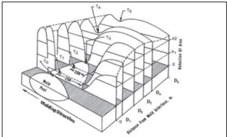
Fig. 6 — Schematic representation of the hot-ductility response of the HAZ.
