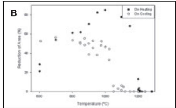
Fig. 11 — Gleeble hot-ductility tests of Alloy IN740. A — Fracture strength; B — reduction of area as a function of testing temperature.
