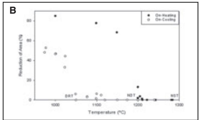
Fig. 3 — Gleeble hot-ductility of Alloy IN740 in the liquation cracking temperature range. A — Fracture strength; B — reduction of area as a function of testing temperature.
