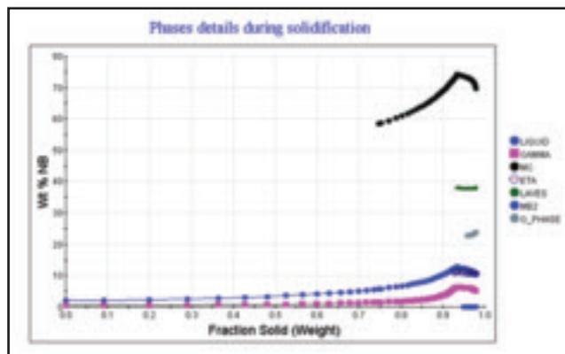
Fig. 9 — Predicted partitioning of Nb into different phases as function of the fraction solid.
