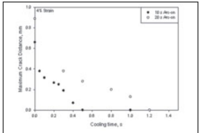
Fig. 4 — Spot-Varestraint testing results of IN740 during the on-heating part of the cycle.
