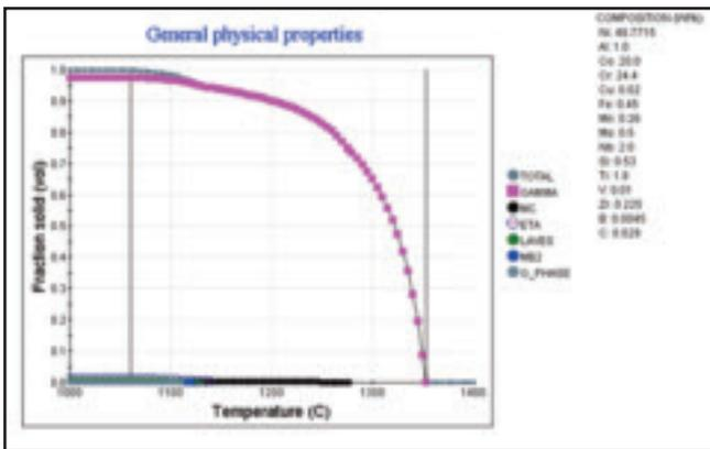
Fig. 10 — Predicted fraction of phases present in the solid as a function of temperature during solidification of the tested IN740 alloy heat.
