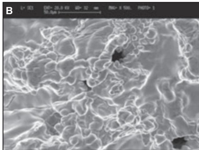
Fig. 7 — A — Example of microfissures observed in cross sections of the IN740 full-size welded joint; B — general fractographic characteristics of Gleeble on-cooling hot-ductility sample showing the presence of liquated phase remaining in the fracture surface.
