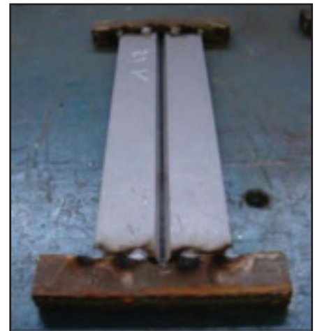
Fig. 2 — Armor steel plates were prepared using V- and double-V-groove welding geometries.
