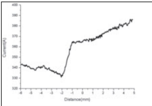
Fig. 7 — Peak currents for the bevel angle of 30 deg.
