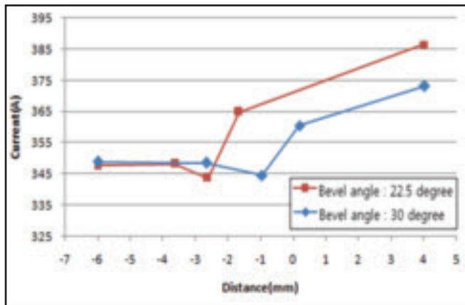
Fig. 8 — Characteristic peak current at various electrode positions for the bevel angles of 22.5 and 30 deg.
