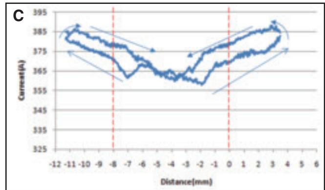
Fig. 10 — Peak current waveforms for 60-deg groove angle. A — 3-mm root opening; B — 5-mm root opening; C — 8-mm root opening.
