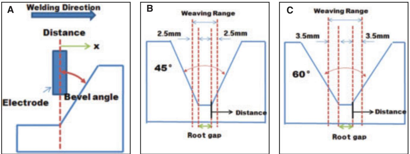
Fig. 3 — Configuration of single bevel and V-groove workpiece. A — Single bevel; B — groove angle of 45 deg; C — groove angle of 60 deg.
