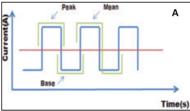
Fig. 1 — Typical shape of pulse signal. A — Types of welding current; B — measured pulse signal.
