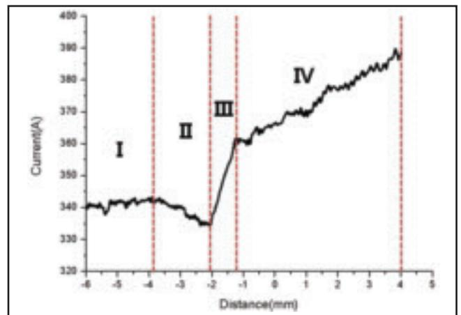
Fig. 5 — Peak currents for the bevel angle of 22.5 deg.
