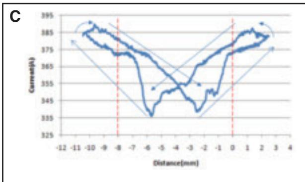
Fig. 9 — Peak current waveforms for 45-deg groove angle. A — 3-mm root opening; B — 5-mm root opening; C — 8-mm root opening.
