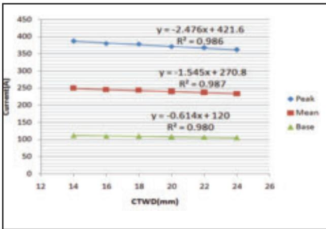
Fig. 4 — Arc sensor sensitivities for pulse parameters.
