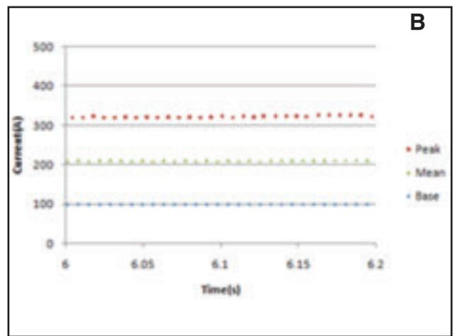
Fig. 2 — Various current signals of pulse GMAW. A — Separated pulse signal; B — moving averaged signal.
