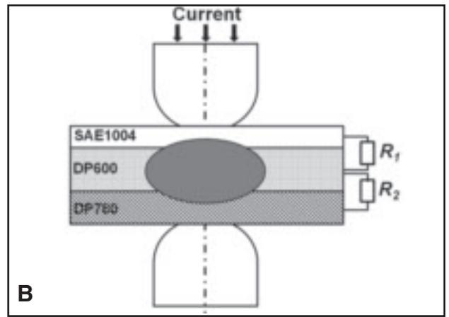
Fig. 8 — Measurement of dynamic resistance between the workpieces. A — Test setup; B — dynamic resistance  $R_1$  and  $R_2$  between the workpieces.
