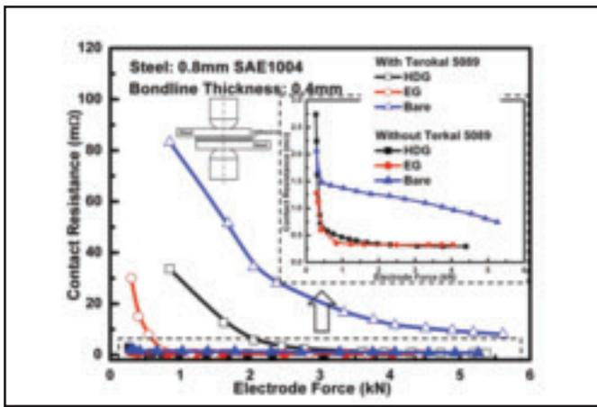
Fig. 5 — Effect of the coating on the static contact resistance in resistance welding and weld-bonding 0.8-mm-thick SAE1004 steel.
