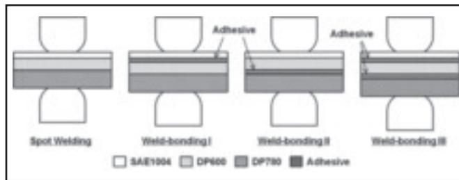
Fig. 2 — Various adhesive locations in weld-bonding three sheets.
