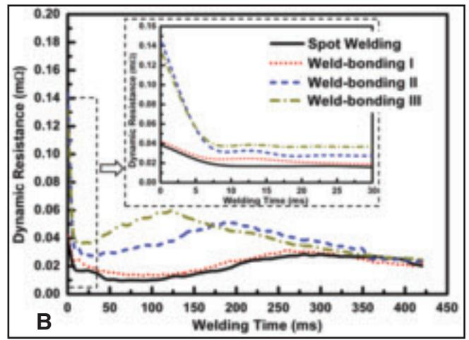
Fig. 9 — Dynamic resistances between workpieces during weld-bonding. A —  $R_1$  between the top and middle sheets; B —  $R_2$  between the middle and bottom sheets.
