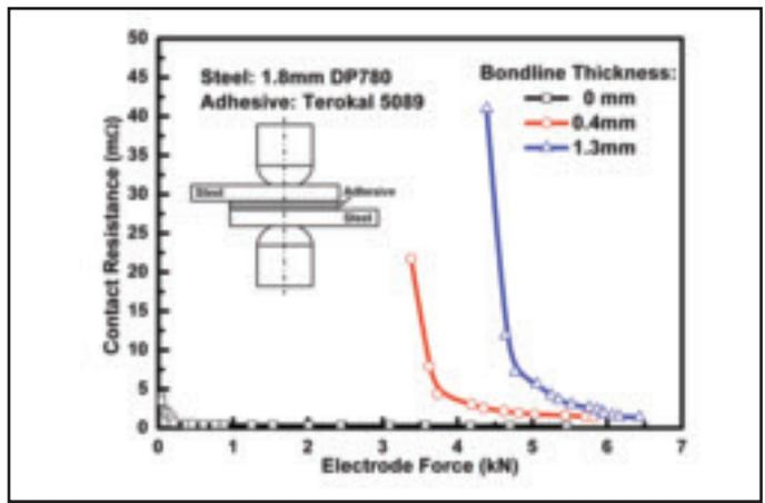
Fig. 6 — Effect of adhesive bondline thickness on the static contact resistances in weld-bonding 1.8-mm-thick DP780 steel.
