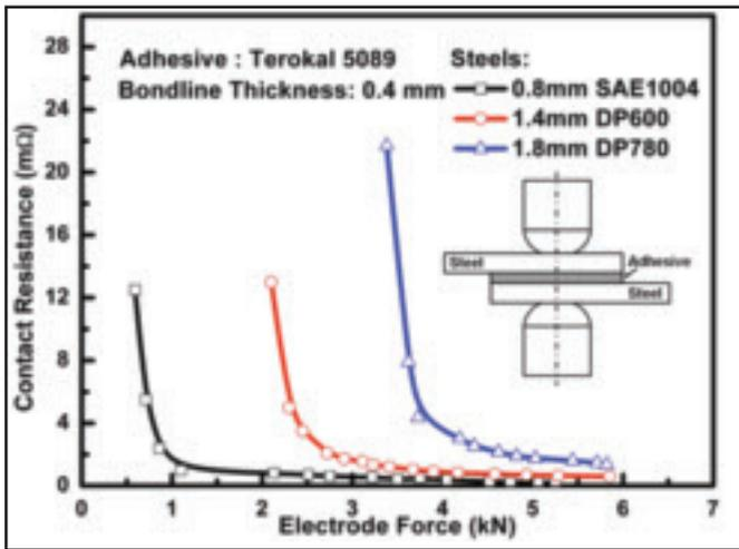
Fig. 7 — The static contact resistances of 0.8-mm-thick SAE1004, 1.4-mm-thick DP600, and 1.8-mm-thick DP780 in weld bonding.
