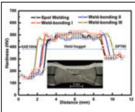
Fig. 13 — Effect of adhesive location on the hardness in weld-bonding multiple workpieces.
