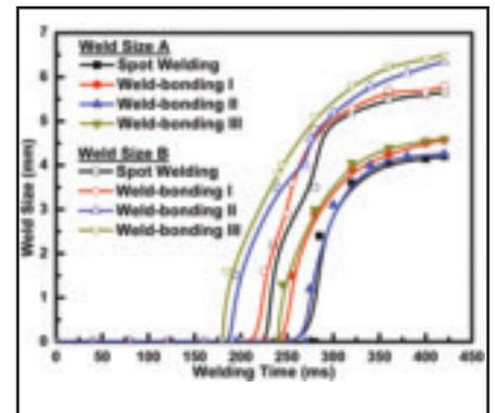
Fig. 10 — Weld formation for different types of weld bonding.
