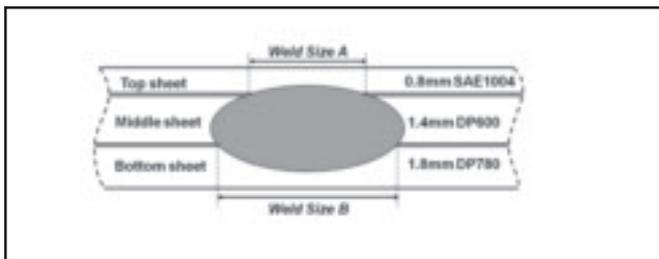
Fig. 1 — Weld nugget configuration in weld-bonding multiple stacks of steels.
