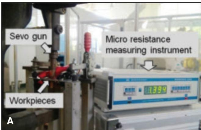
Fig. 3 — Experimental setup for measuring the static contact resistance between the steel sheets and adhesive. A — Test setup; B — resistances between the steel sheets.
