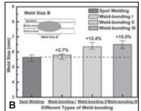
Fig. 14 — Effect of adhesive location on the weld size. A — Weld size A; B — weld size B.
