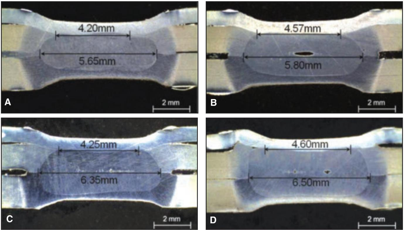
Fig. 12 — Effect of adhesive placement on the weld size. A — No adhesive (spot welding); B — weld-bonding type I; C — weld-bonding type II; and D — weld-bonding type III.
