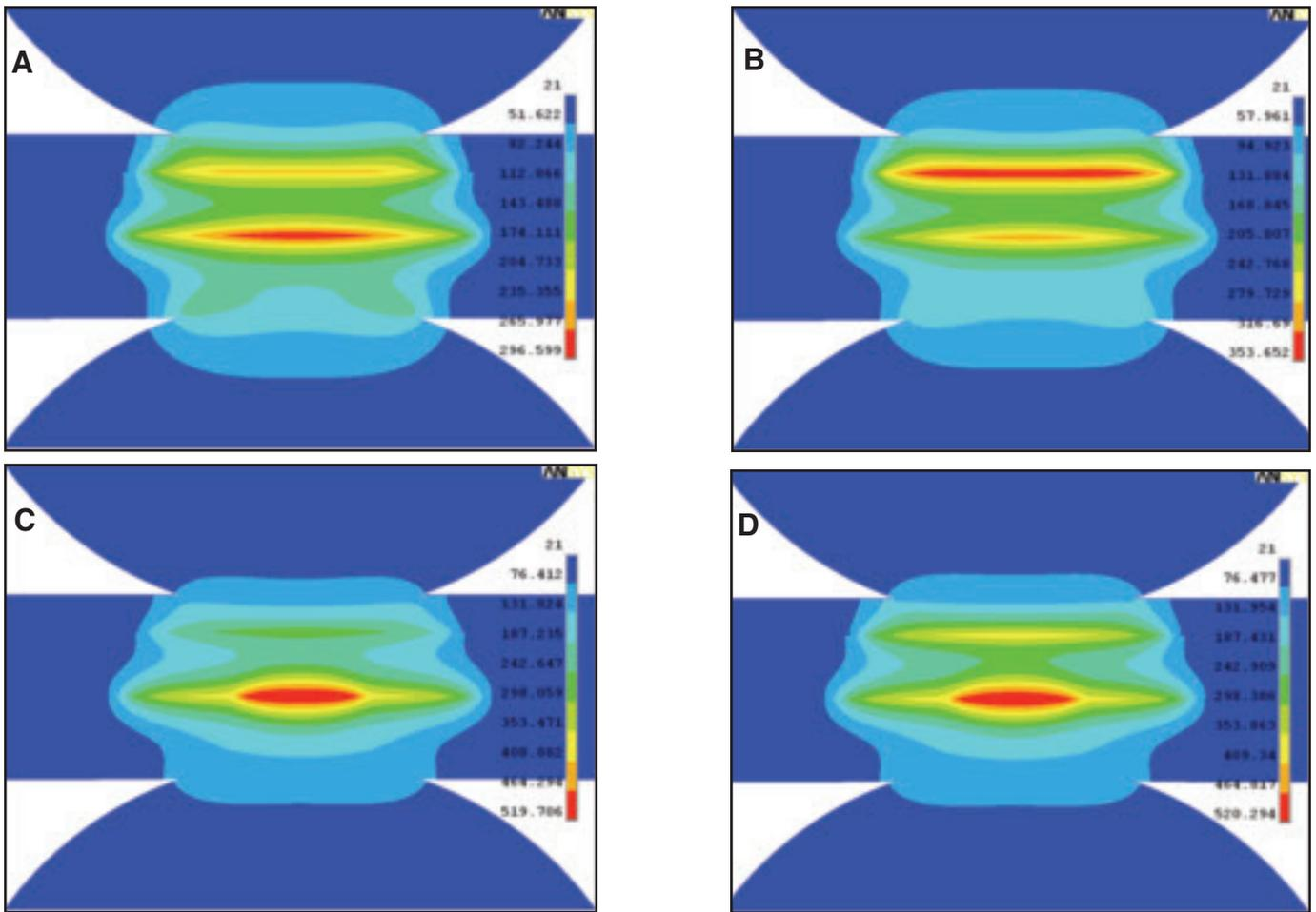
Fig. 11 — Initial temperature distributions with different adhesive locations. A — Spot welding; B — weld-bonding I; C — weld-bonding II; and D — weld-bonding III (welding time = 20 ms).
