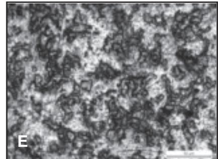
Fig. 4 — Effect of adhesive on the contact state in weld-bonding 0.8-mm-thick galvanized SAE1004 steel. A — Contact area between workpieces after squeezing; B — residual adhesive between the workpieces; C — contact area without adhesive; D — enlarged view of area 1 in B; and E — enlarged view of area 2 in C.
