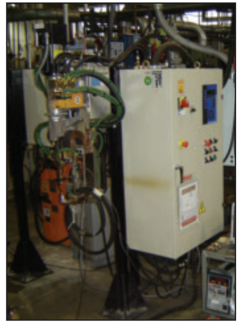
Fig. 13 — ARO electric servo-gun with MFDC power supply.
