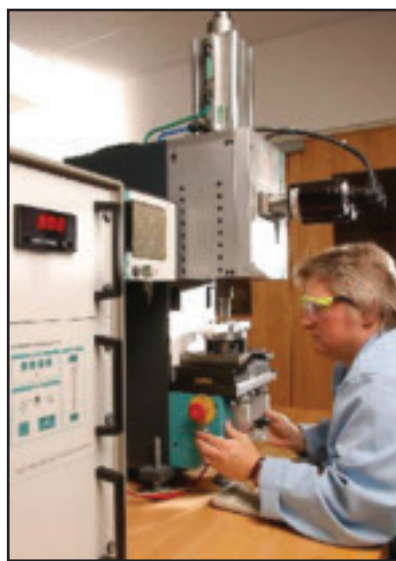
Fig. 34 — Configurations of torsional welding systems for ultrasonic spot welding. A — Schematic representation of the torsional ultrasonic welding configuration; B — actual 10-kW torsional welding system at Edison Welding Institute.
