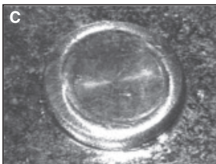
Fig. 26 — Morphological details of a clinch joint between sheet materials. A — Clinch joint cross section; B — top view of the clinch joint; C — root view of the clinch joint.
