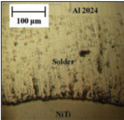
Fig. 10 — USS NiTi/Al 2024 USS lap joint cross section.
