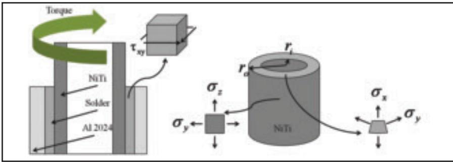
Fig. 9 — Differential solder element in USS torsion joint.
