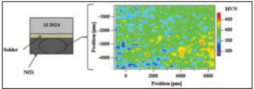
Fig. 11 — Hardness map of NiTi/Al 2024 USS lap joint.
