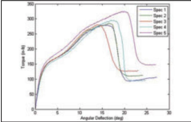
Fig. 7 — Torque-angle plots of NiTi/Al 2024 USS torsion joints.
