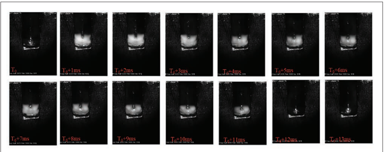
Fig. 11 — High-speed images of NGHW ( D = 3 mm).
