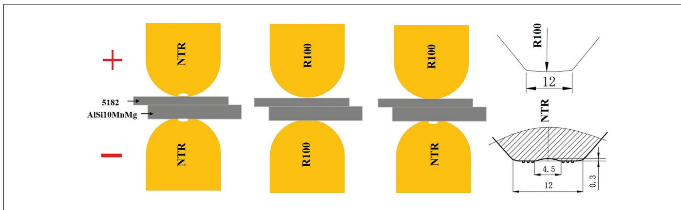
Fig. 1 — The welding conditions and structure of the three types of electrode combinations.
