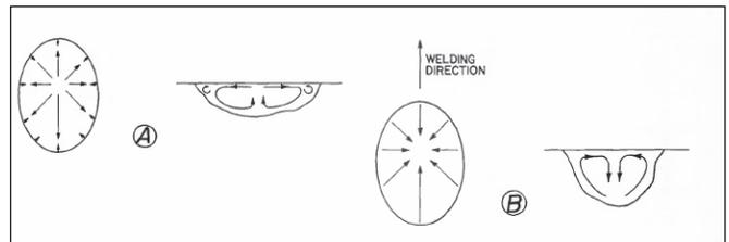
Fig. 3 — Apparent fluid flow pattern on weld pool surface and proposed subsurface flow pattern: A — High-aluminum welds; B — high-sulfur welds.
