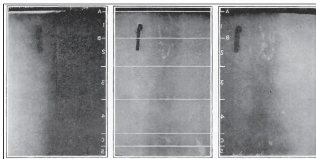
Fig. 1 — Images of some of the first use of x-rays to detect weld discontinuities and defects.
