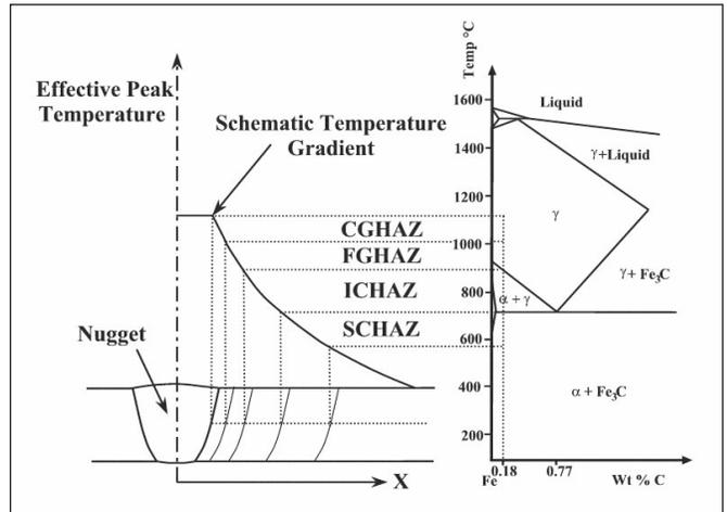
Fig. 4 — Schematic illustration of the different regions of the HAZ of a friction stir weld on mild steel and their relation to effective temperatures in the Fe-Fe<sub>3</sub>C binary system.
